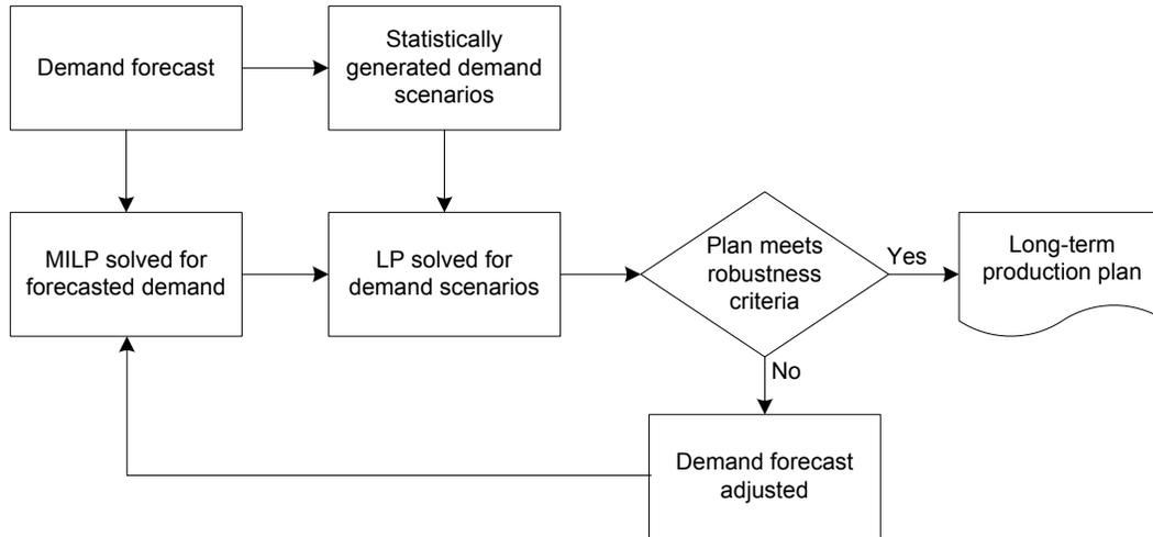
Figure 1: Flowchart explaining the structure of the iterative procedure. Each component is further explained in the following sections.
