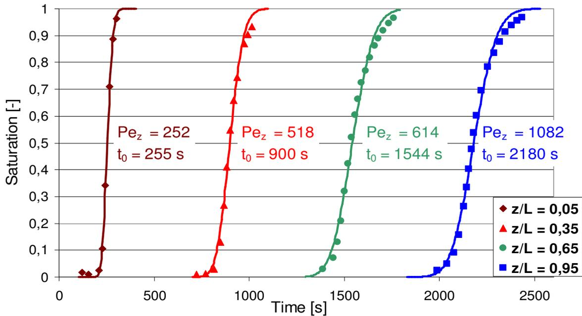
Figure 3: Experimental (points) and fitted breakthrough curves (lines) at different axial positions  $z/L$
