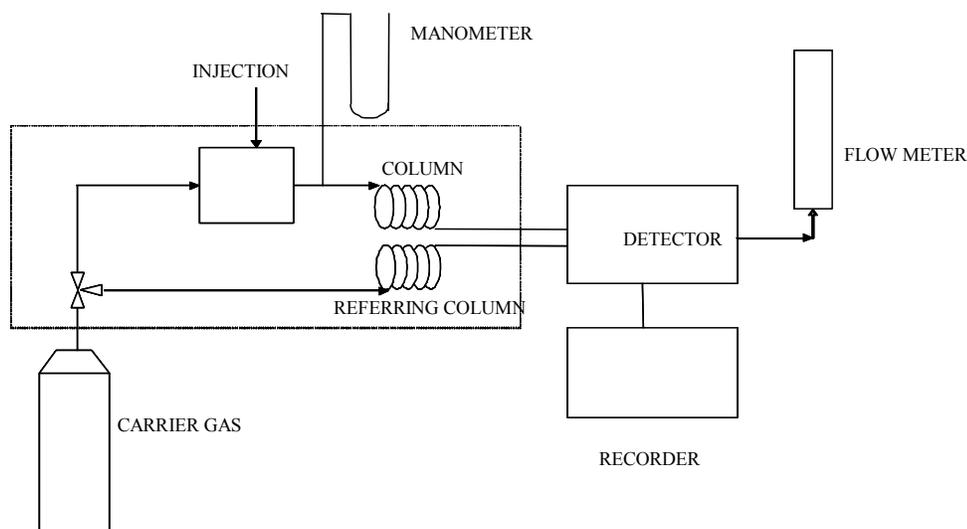
**Fig. 6:** Experimental apparatus adopted for IGC measurements.
