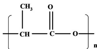
**Fig. 3:** L and DL-PLA molecular structure.
