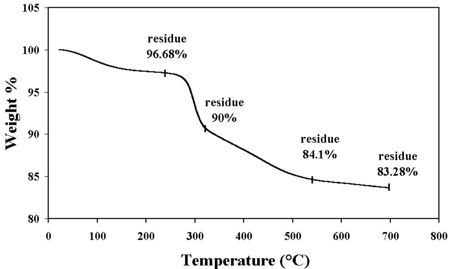
Typical thermo-gravimetric analysis results of the simulant formulation.
