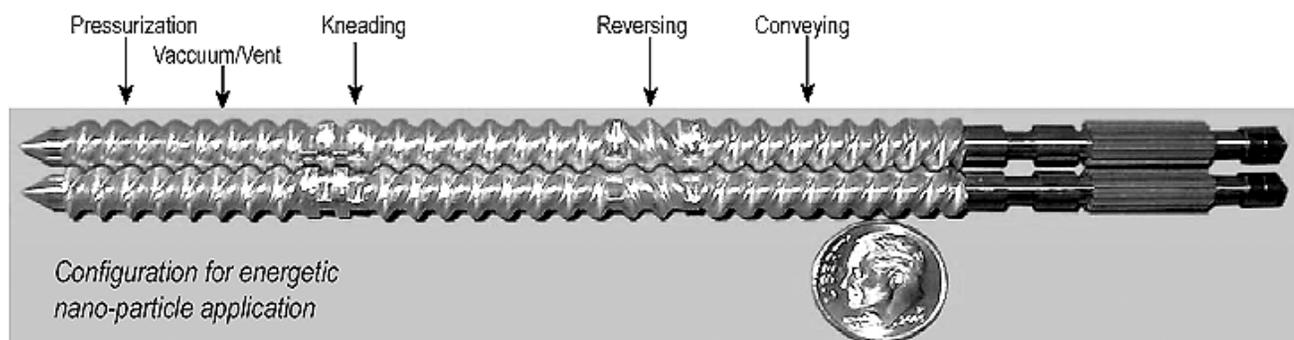
Twin screw extruder specifically designed and built for incorporating nanoparticles.
