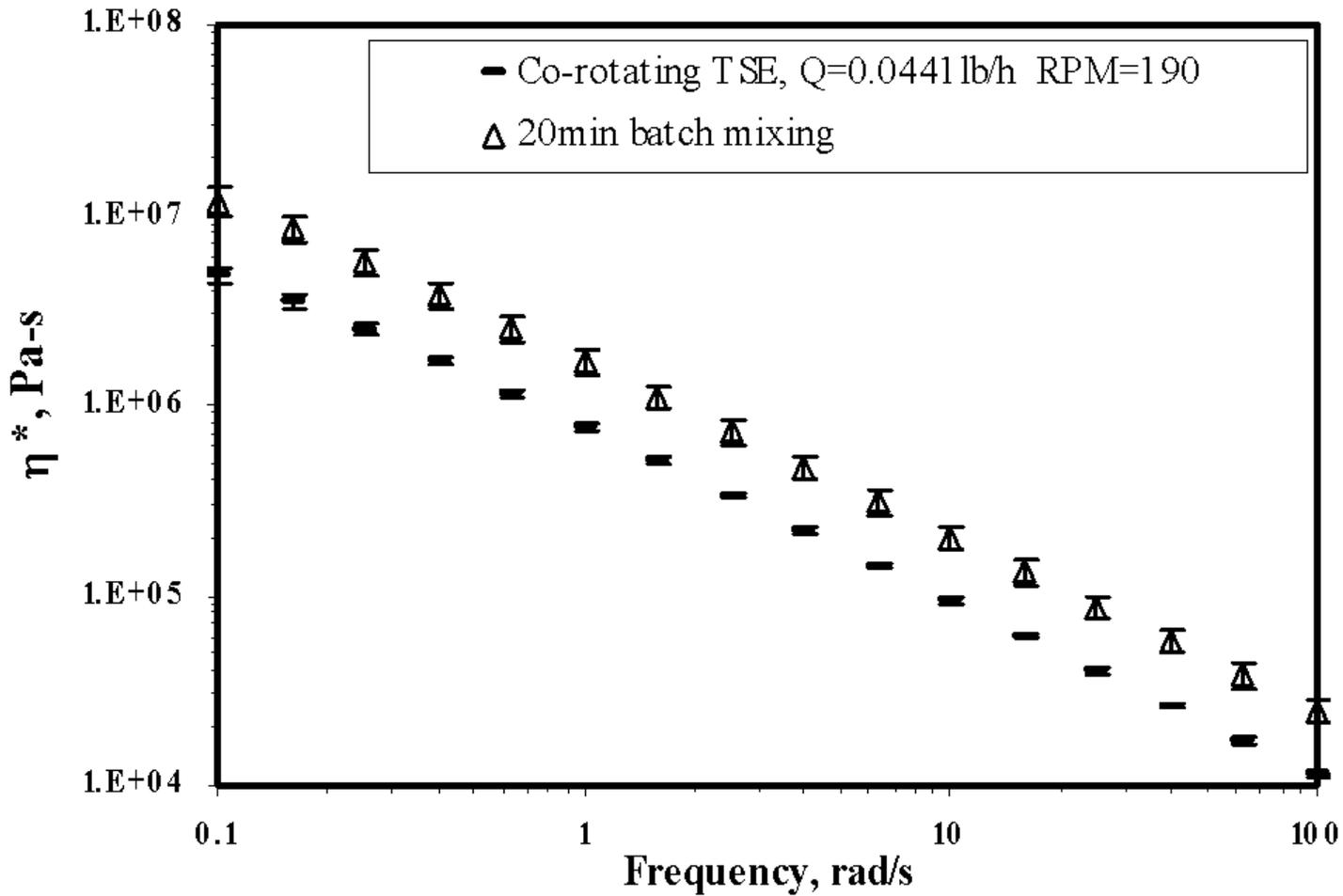
Confidence intervals of the magnitude of complex viscosity,  $\eta^*$ , data for mixtures prepared with conventional and twin screw extrusion processes
