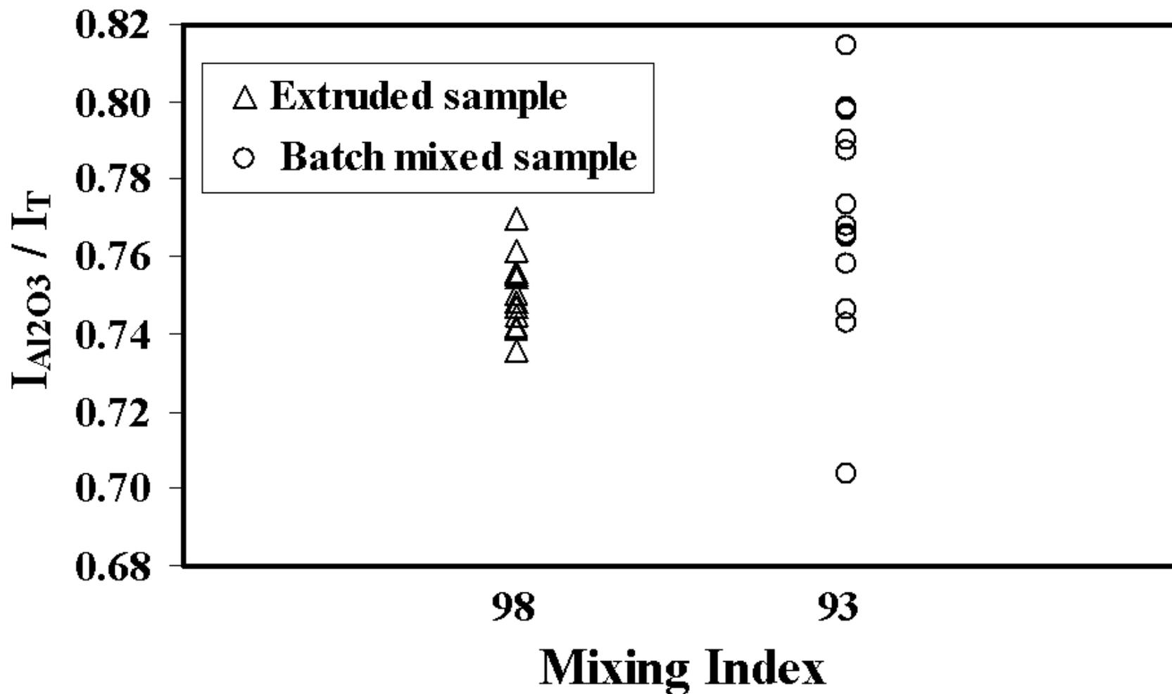
Scatter of the x-ray diffraction data for mixtures prepared with conventional and twin screw extrusion processes and their mixing indices
