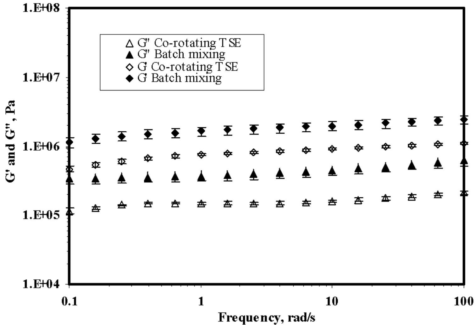
Confidence intervals of the storage modulus,  $G'$ , and loss modulus,  $G''$ , data for mixtures prepared with conventional and twin screw extrusion processes
