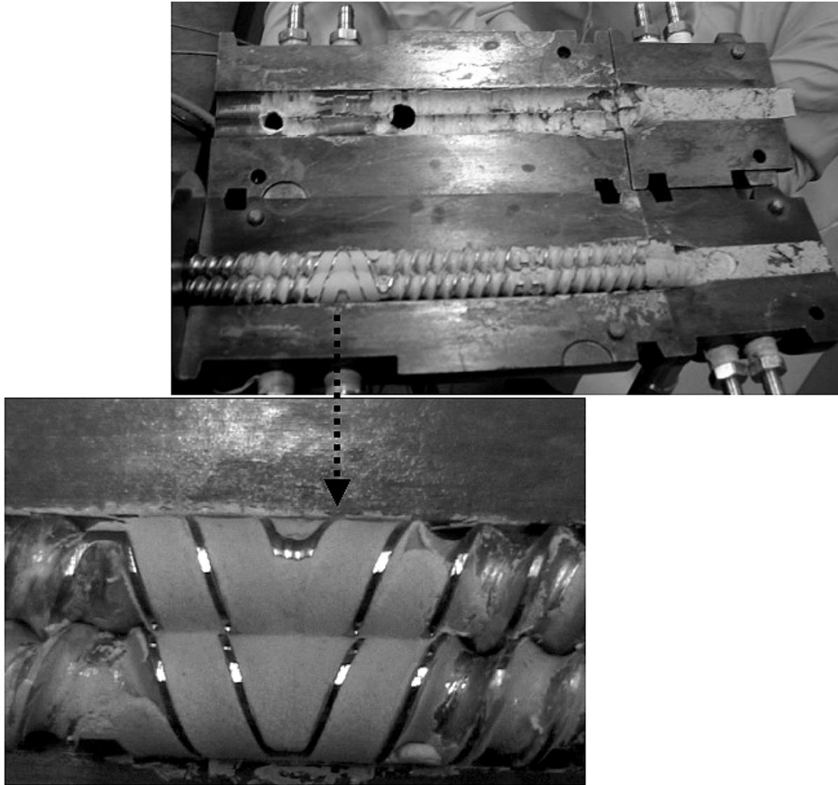
The typical degree of fill distributions in the twin screw extruder upon a dead stop.
