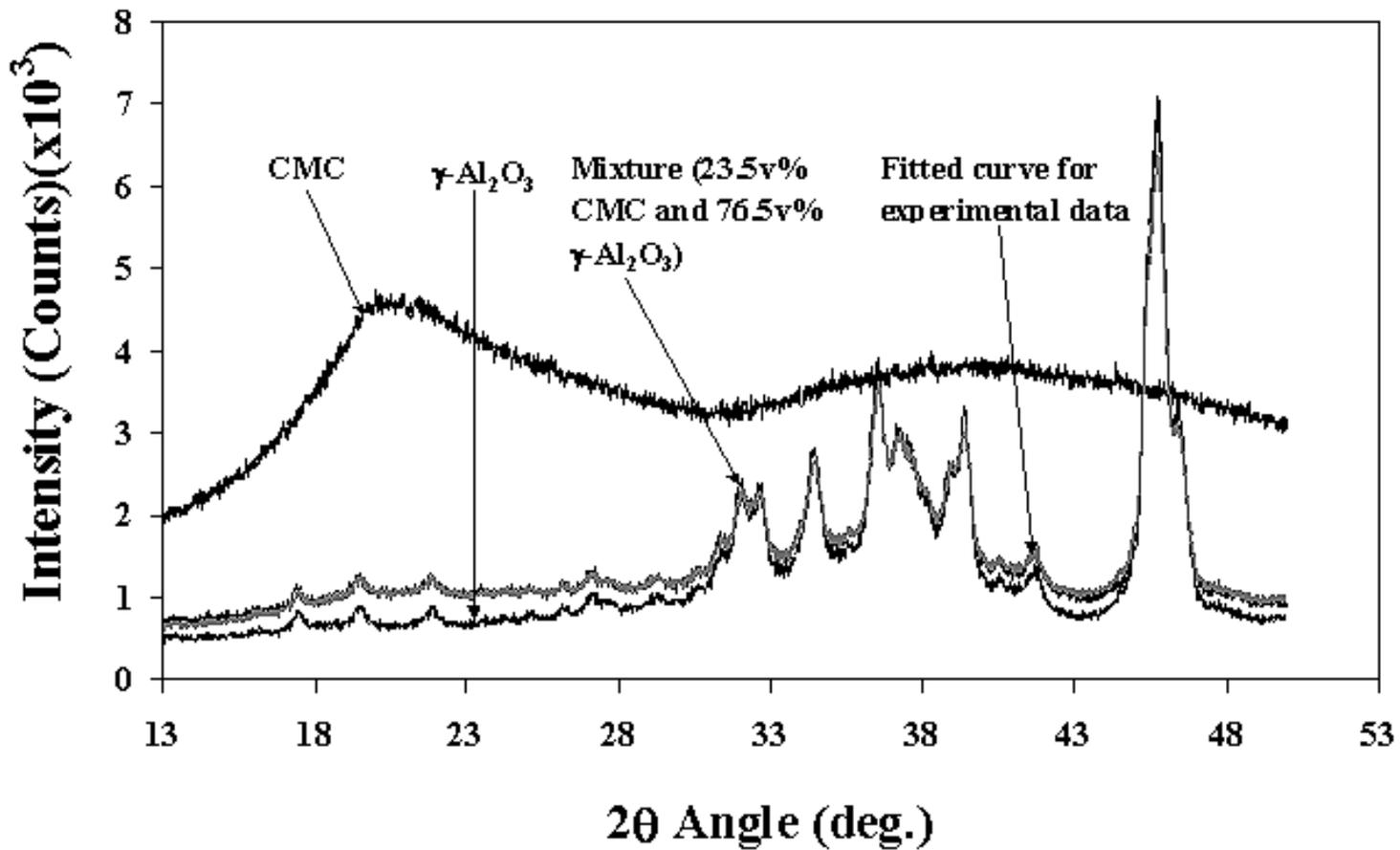
Typical x-ray diffraction patterns of the simulant formulation and its various ingredients.
