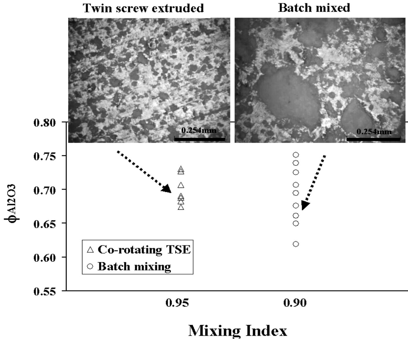
Scatter of the thermo-gravimetric analysis data for mixtures prepared with conventional and twin screw extrusion processes and their mixing indices
