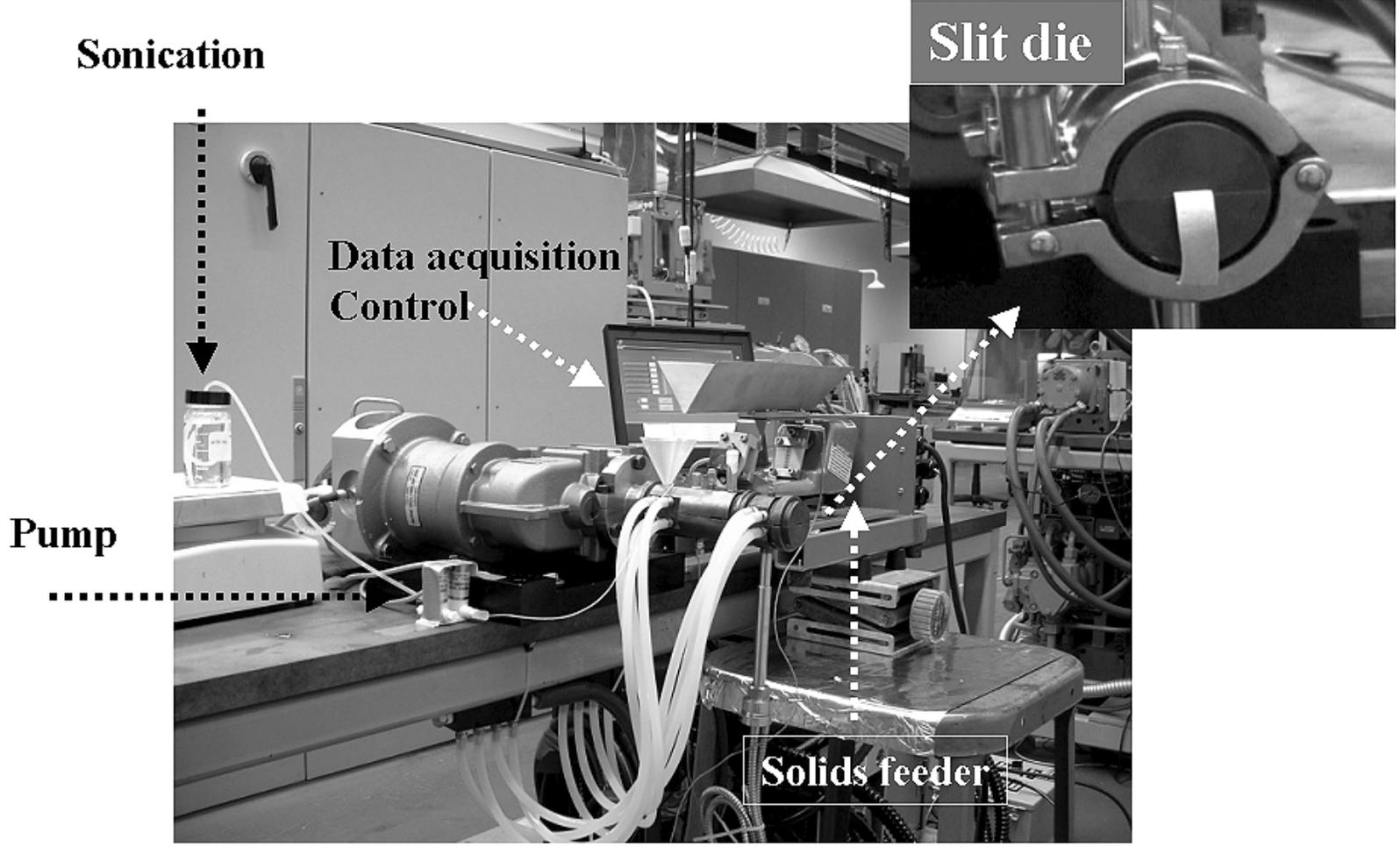
The auxiliaries of the twin screw extruder specifically designed and built for incorporating nanoparticles
