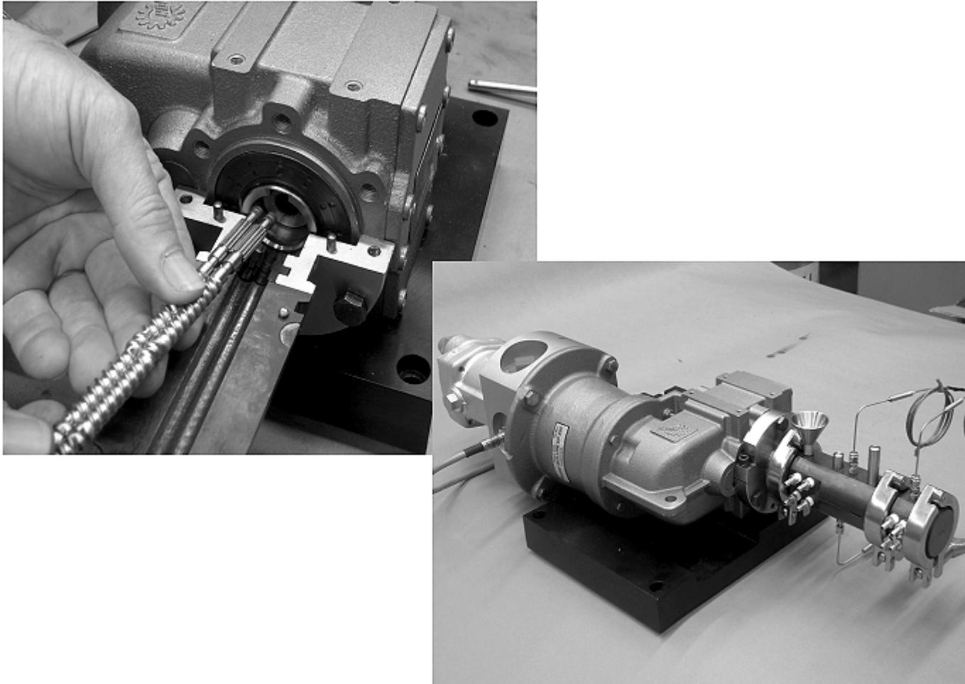
Mini extruder specifically designed for processing of nanoenergetics
