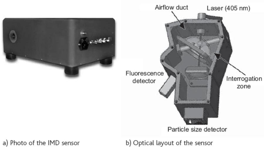
*Fig. 2 Model IMD-A airborne microbial sensor*
