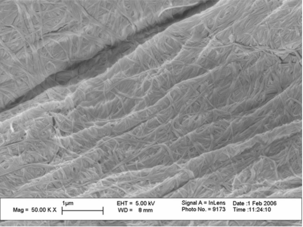
Figure 2 Scanning electron microscopy of hemp fibre after bacterial cellulose grafting
