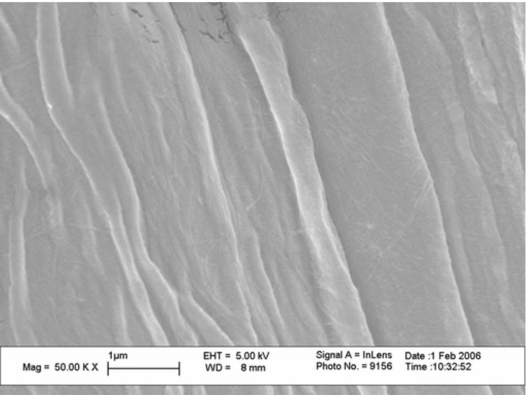
Figure 1 Scanning electron microscopy of hemp fibre
