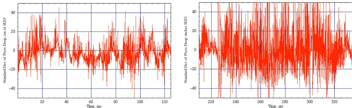
Figure 4: Standard deviation of the pressure drop signal without (left) and with (right) the presence of gas bypassing in the 0.9 meter diameter fluidized bed.
