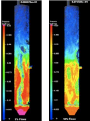
Figure 10: Barracuda™ simulations of a fluidized bed containing 4% (left) and 12% (right) fines.
