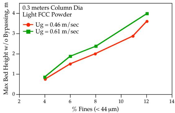
Figure 8: Minimum bed height needed to prevent gas bypassing with respect to fines concentration and superficial gas velocity in the 0.3 meter diameter unit with light FCC powder.
