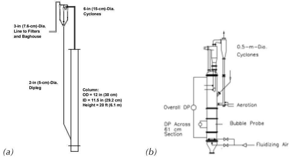
Figure 2: Schematics of the (a) 0.3 meter diameter by 6.1 meter and the (b) 0.9 meter diameter by 6.1 meter fluidized bed test units.
