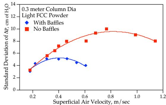
Figure 9: Gas bypassing, as indicated by pressure fluctuations, of a fluidized bed with (red) and without (blue) horizontal baffles at various superficial gas velocities.
