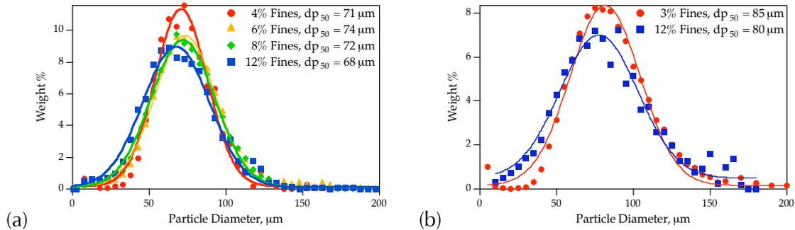
Figure 3: Particle size distribution of (a) light FCC powder with 4, 6, 8 and 12% fines, and (b) heavy FCC powder with 4 and 12% fines.
