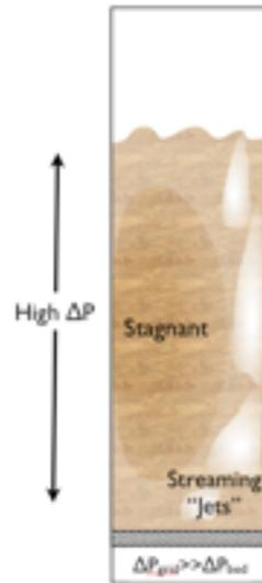
Figure 1: Illustration of the gas bypassing concept in a large fluidized bed.
