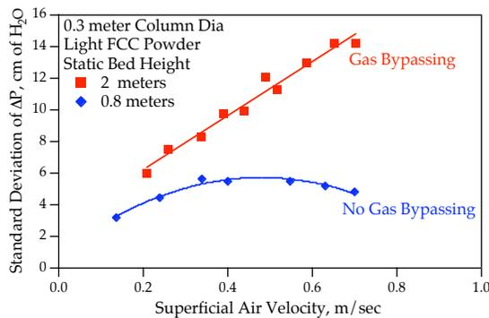
Figure 6: Pressure fluctuations, as an indication of gas bypassing, with respect to superficial gas velocities for a fluidized bed of light FCC powder (6% fines) with a bed height of 0.8 and 2.0 meters in the 0.3 meter diameter fluidized bed unit.
