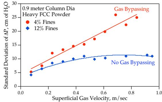
Figure 7: Pressure fluctuations, as an indication of gas bypassing, with respect to superficial gas velocities for a fluidized bed of heavy FCC powder with a fines content of 3 to 12% in the 0.9 meter diameter fluidized bed unit.
