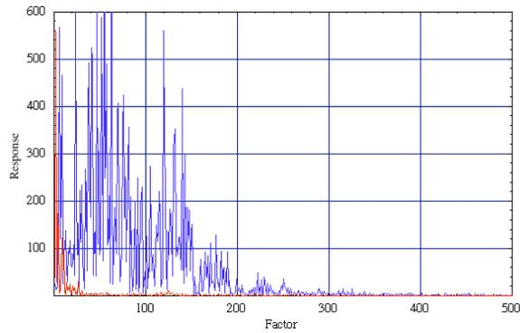
Figure 5: Power spectrum analysis with Hanning filtering for a pressure response curve (Figure 4) indicative of a fluidized bed with (blue) and without (red) gas bypassing.
