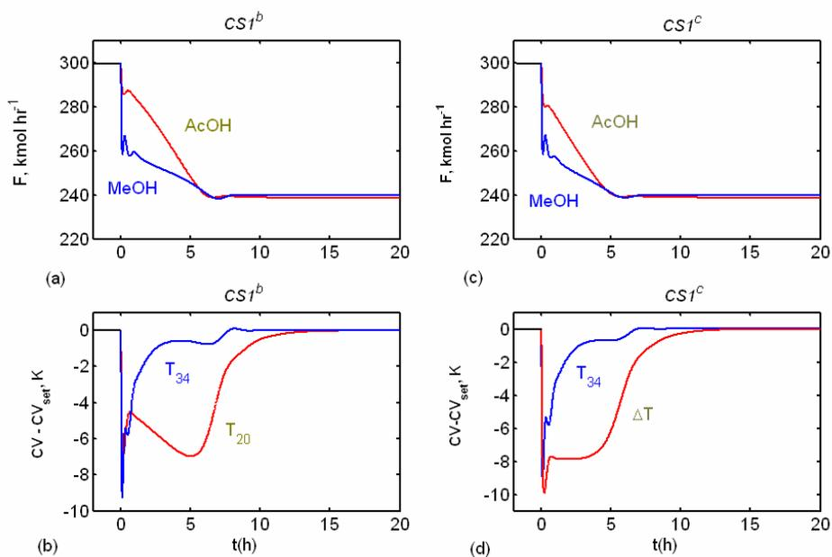
Fig. 10. Manipulated and controlled variable dynamic response for  $-20\%$  change in reboiler duty for  $CS1^b$  and  $CS1^c$ .
