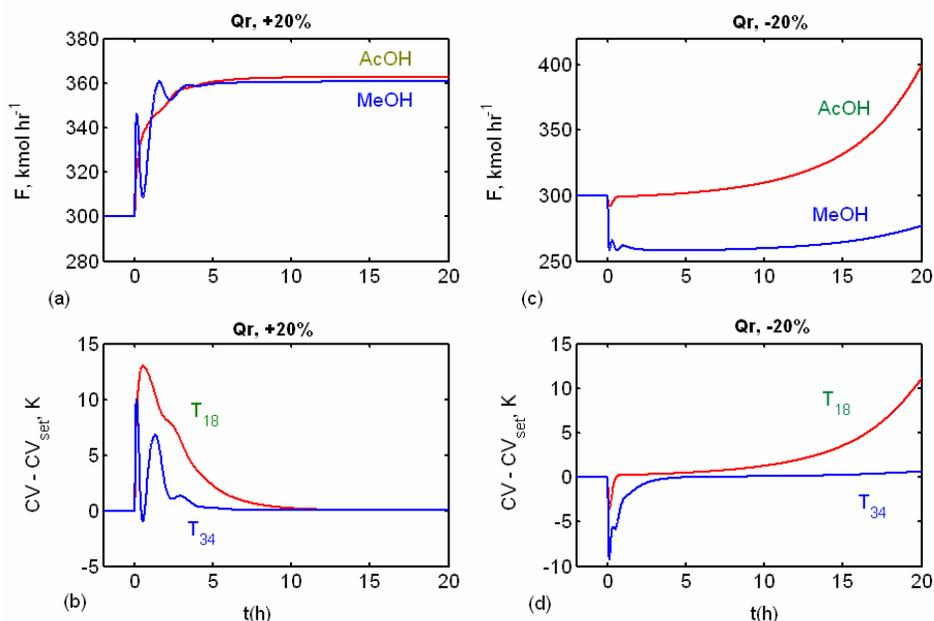
Fig. 9. Dynamic response of manipulated and control variables for  $\pm 20\%$  change in reboiler duty for  $CS1^a$  control structure.
