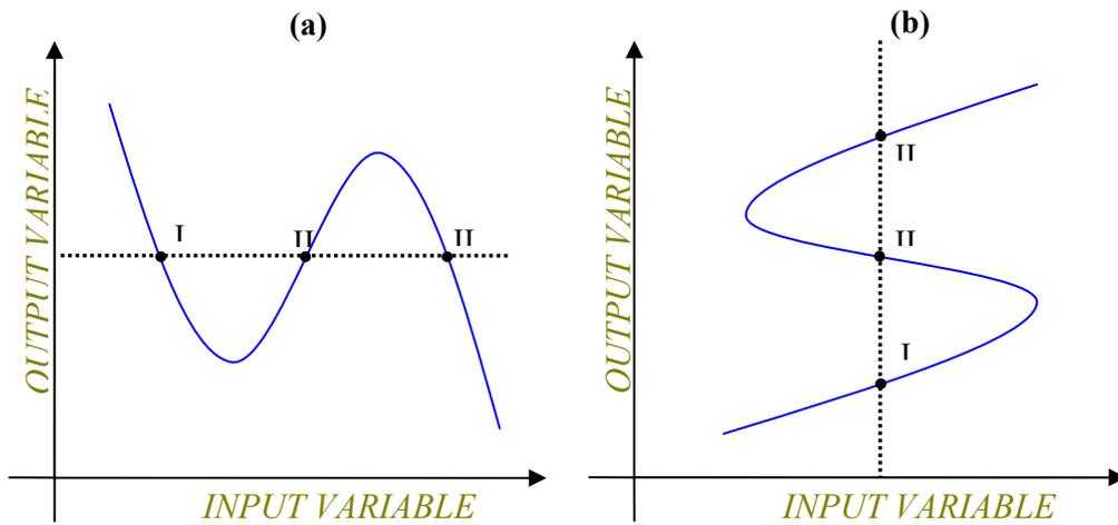
Fig. 1. Two types of steady-state multiplicities
