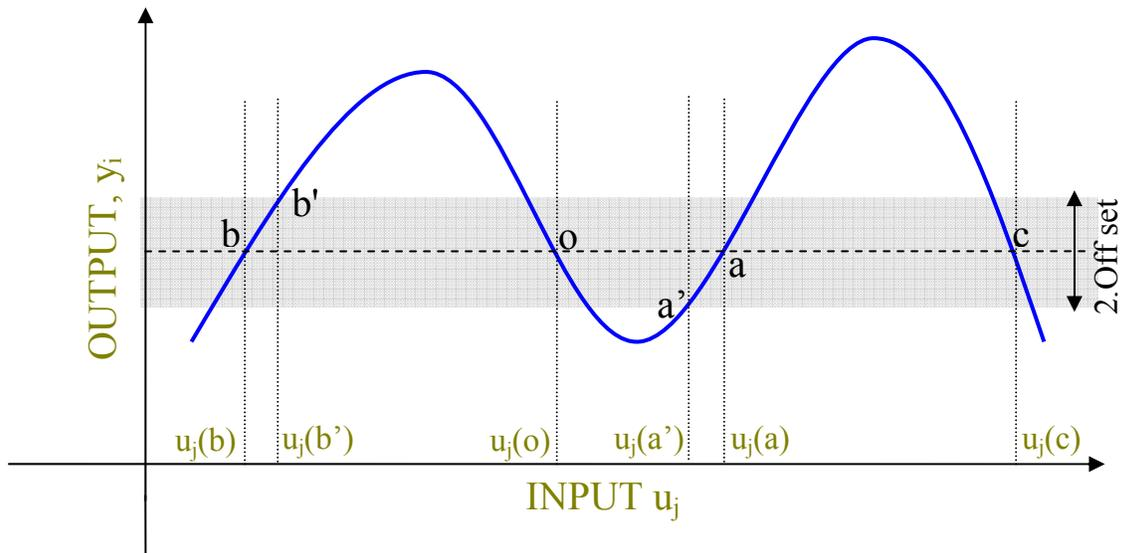
Fig. 2. A non-linear input-output relation with input multiplicity
