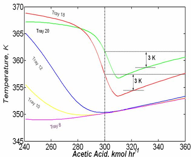
Fig. 6. Variation of reactive tray temperatures with respect to acetic acid.
