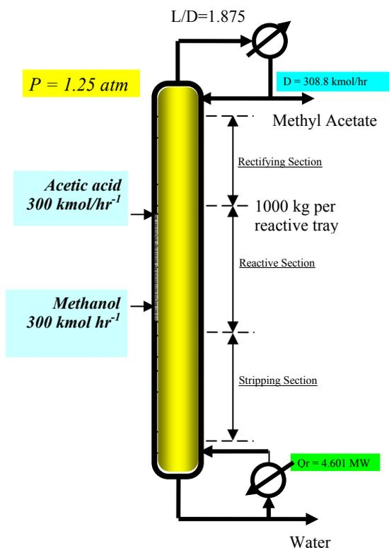
Fig. 3. Schematic of methyl acetate RD column
