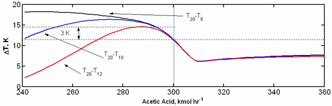
Fig. 7. Steady-state variation of difference between two reactive tray temperatures with Acetic acid
