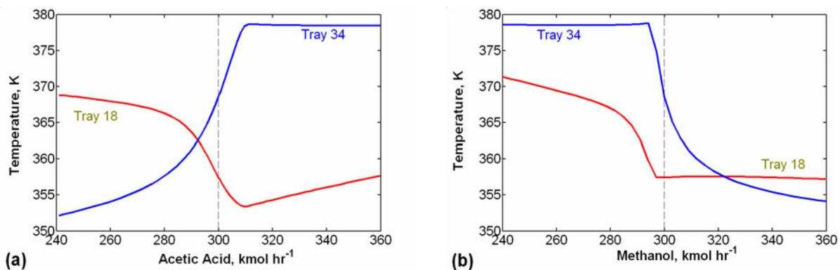
Fig. 4. Steady-state input-output relation of Tray 18 and Tray 34 temperatures.
