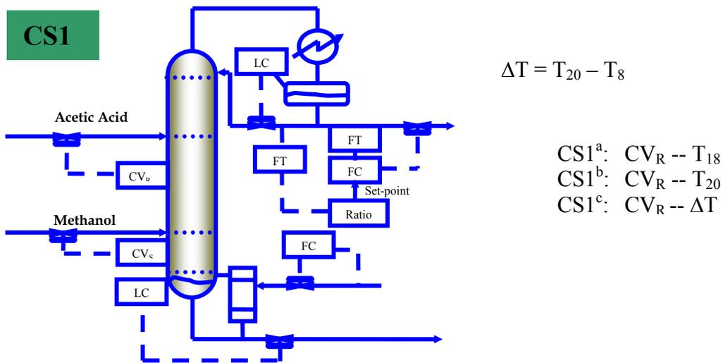
Fig. 8. Schematic of candidate control structures CS1 and CS2
