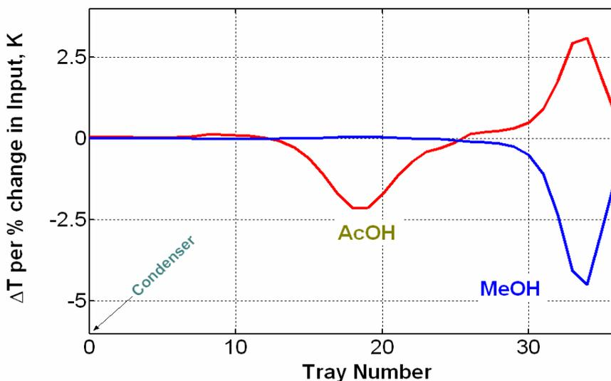
Fig. 4. Tray temperature sensitivities with respect to acetic acid (AcOH) and methanol (MeOH).
