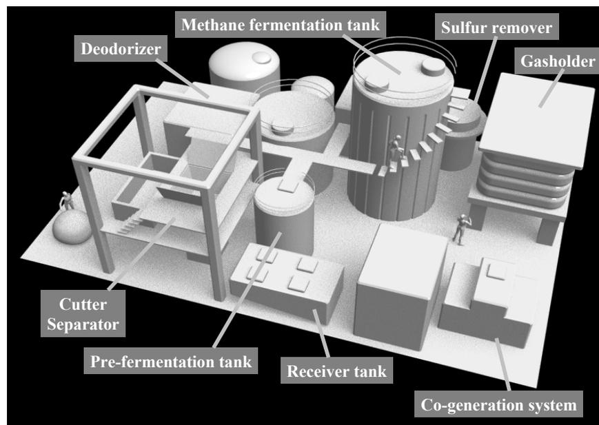
**Figure 7** Layout of the plant
