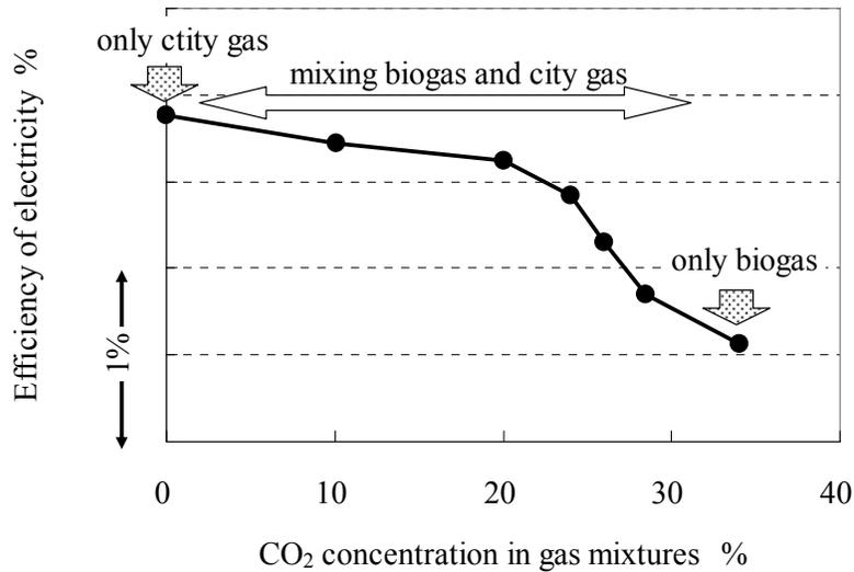
**Figure 11** Results of the gas engine test
