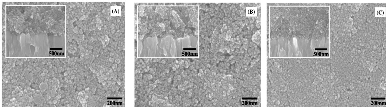
**FIG. 5** FE-SEM images of the vertical cut of photoelectrodes with the concentration of acetic acid treated TiO<sub>2</sub> (inlet) and photoelectrode surface images
