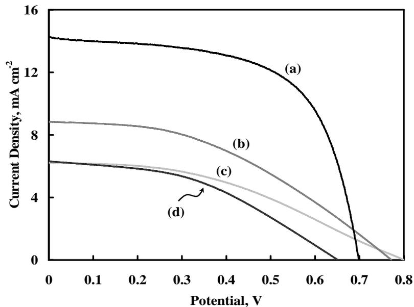
**FIG. 3** Photocurrent-photovoltaic (J–V) characteristics of acid treated  $\text{TiO}_2$  nano particles of DSSCs (a)  $\text{CH}_3\text{COOH}$ , (b)  $\text{HCl}$  (c) None acid and (d)  $\text{H}_2\text{SO}_4$
