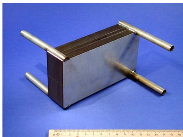
Fig.5: 2 kW Counter-flow 2 kW water-gas shift reactor/heat-exchanger
