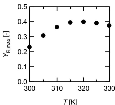
Fig. 3. Relation between  $Y_{R,max}$  and reaction temperature for the reaction system shown in Eq. 1 of  $E_1 = 150$  kJ/mol,  $E_2 = 50$  kJ/mol.  $\phi_0 = 10$ .  $T$  is the fixed temperature.
