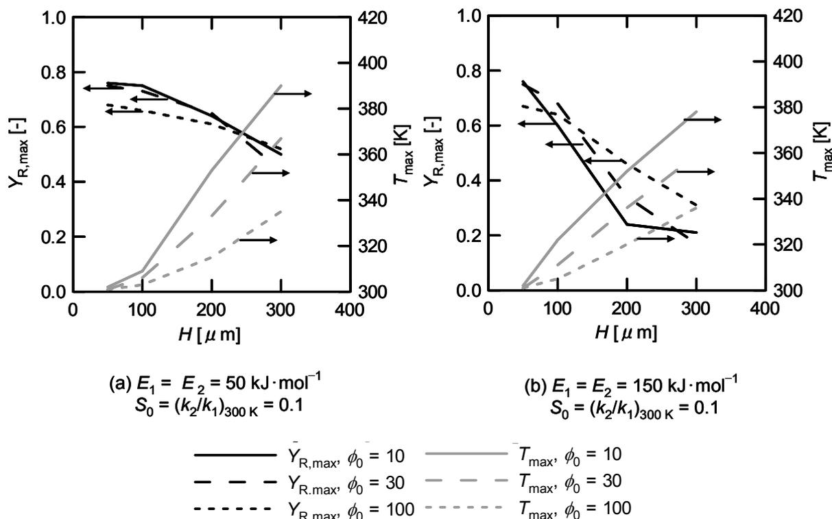
Fig. 2.  $Y_{R,max}$  and  $T_{max}$  in the reactor of each fluid segment size for the two  $E_2/E_1$ . indicate that the effect of decreasing  $k_2/k_1$  dominates that of reaching diffusion controlled
