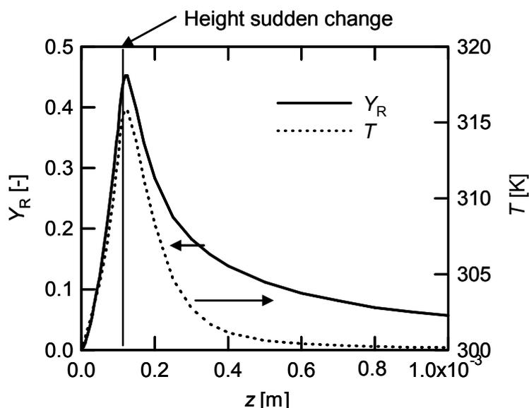
Fig. 5 Profile of  $Y_R$  and  $T$  in the reactor of  $H_1 = 50 \mu\text{m}$ .  $H_2 = 150 \mu\text{m}$ .  $z$  is the axial position.
