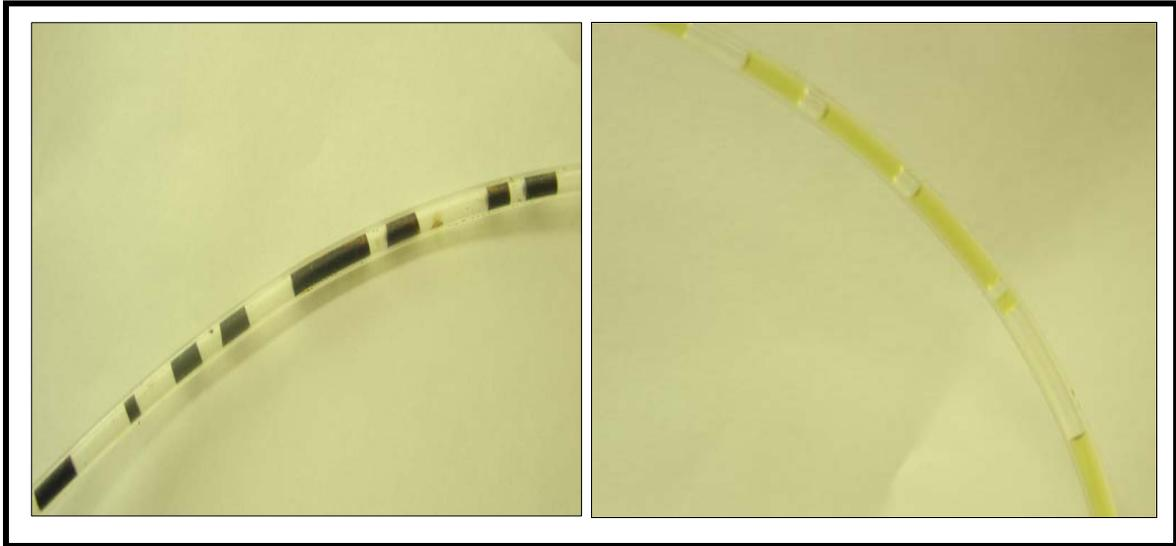
**Figure 6:** Gradual Color Fading of the Produced Oil for GAGD Yates Corefloods
