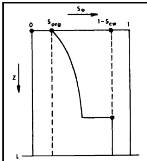
**Figure 5:** Buckley-Leverett Saturation Profile for Stable Downward Displacement (Hagoort, 1980)
