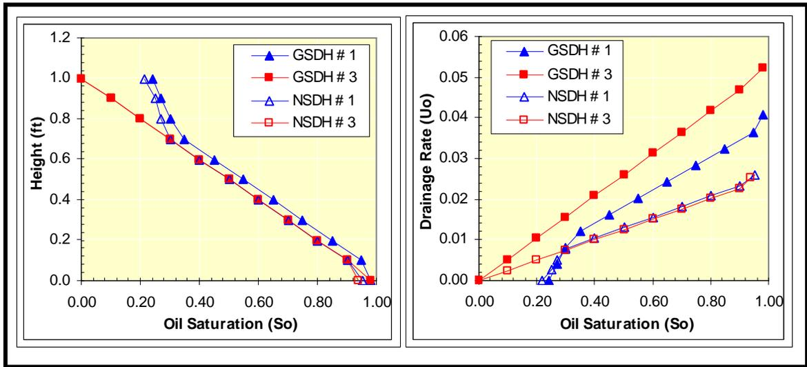
**Figure 1:** R&B Model Predicted Vertical Drainage Rates and Gas Interface Height for Each Core Block
