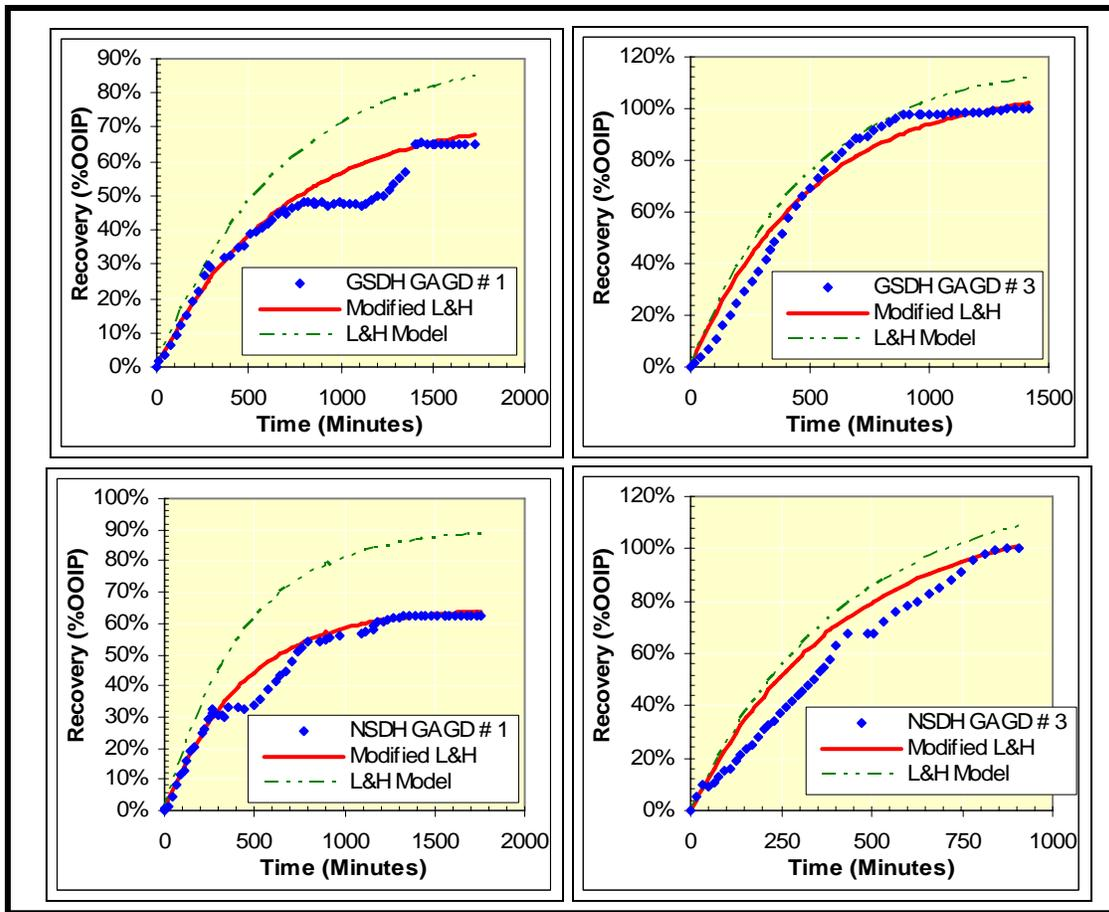
**Figure 4:** Comparison of Experimental and Modified L&H Model Predicted Oil Production Rates for Forced Gravity Drainage 1-D GAGD Corefloods
