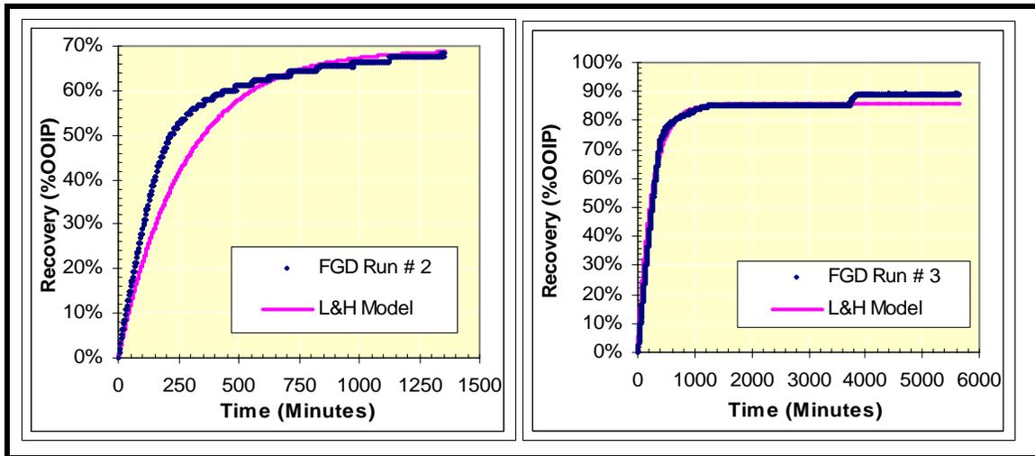
**Figure 2:** Comparison of Experimental and L&H Model Predicted Oil Production Rates for Two Selected Free Gravity Drainage Tests in a 2-D Physical Model
