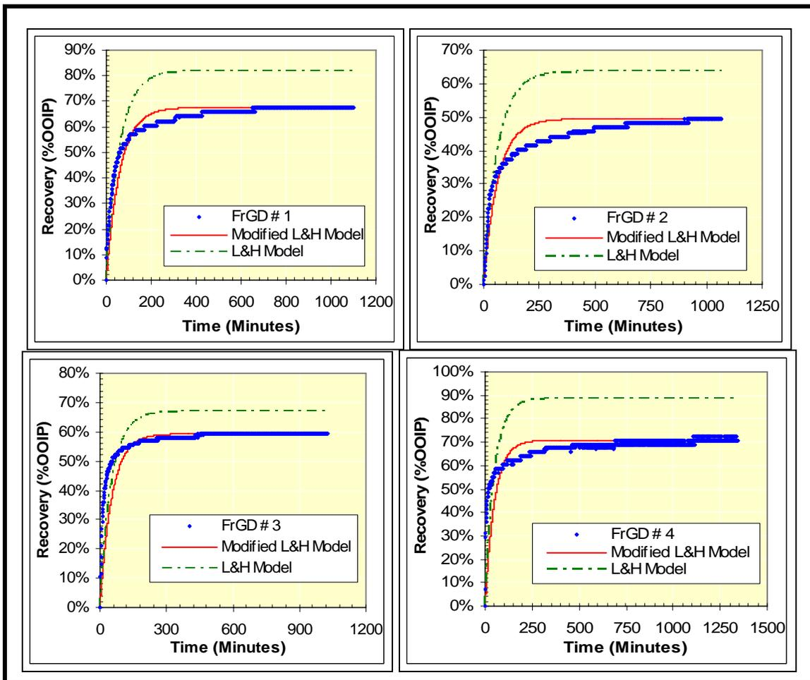
**Figure 3:** Comparison of Experimental, L&H and Modified L&H Models Predicted Oil Production Rates for Forced Gravity Drainage 2-D Physical Model GAGD Floods
