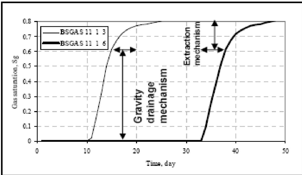
**Figure 7:** Numerical Simulations Demonstrating the Presence of Gravity Drainage Film Flow Mechanism and the Extraction Mechanism in Forced Gravity Drainage (GAGD) Type Flow (Darvish et al., 2004)
