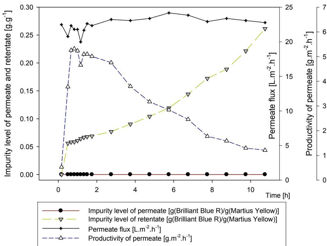
**Figure 4** Constant volume diafiltration (CVDF) testing in a single-stage flowthrough stirred cell at 30 bar, room temperature with STARMEM 228 membrane: Impurity level of permeate and retentate, permeate flux and productivity
