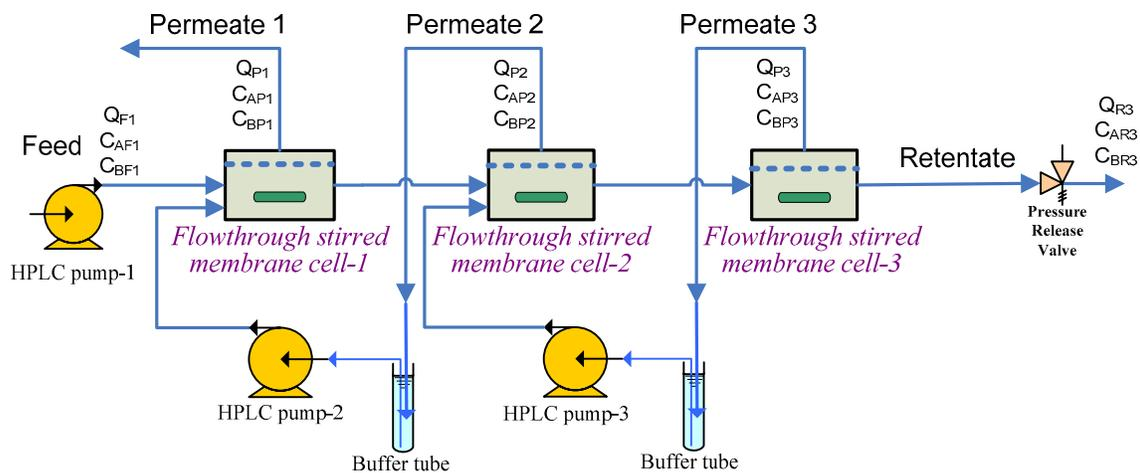
**Figure 1** Schematic of API impurity separation set-up in a three-stage membrane cascade (fed to the first cell, permeate recycling configuration)
