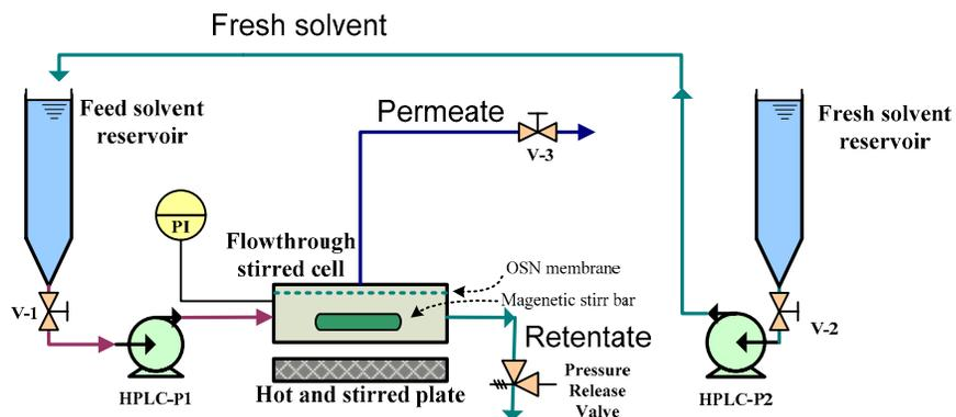
**Figure 2** Schematic of API impurity separation set-up in a single-stage flowthrough stirred membrane cell for constant volume diafiltration (CVDF) testing
