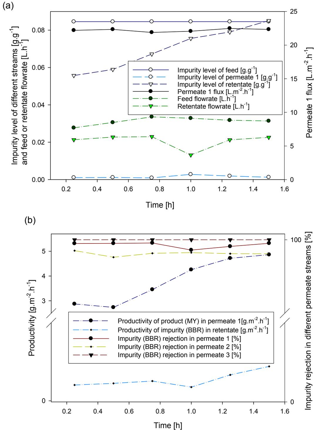
**Figure 3** API impurity separation results in a three-stage membrane cascade (fed to the first cell, permeate recycling configuration) at 30 bar, room temperature with STARMEM 228 membrane: **(a)** Impurity level in different streams, feed and retentate flowrates and permeate 1 flux; **(b)** Productivity and impurity rejections in different streams
