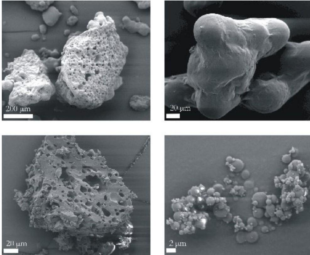
Figure 1: Particles dried using the PGSS-Drying process
