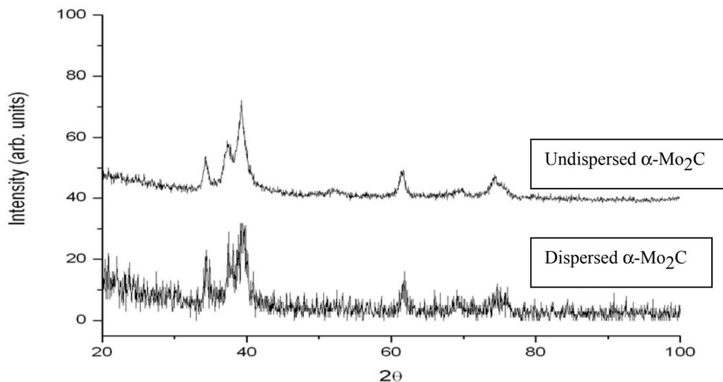
**Figure 2:** XRD analysis of Undispersed and Dispersed  $\alpha\text{-Mo}_2\text{C}$  nanocrystallites
