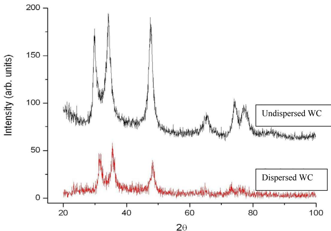
**Figure 5:** XRD Analysis of Undispersed and Dispersed WC Nanocrystallites
