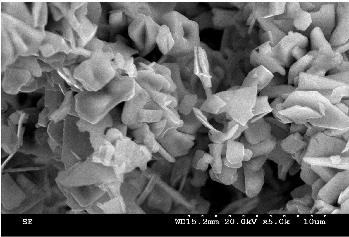
Figure 3: SEM of Undispersed  $\alpha$ -Mo<sub>2</sub>C at 10  $\mu$ m Scale and 5,000 Magnification
