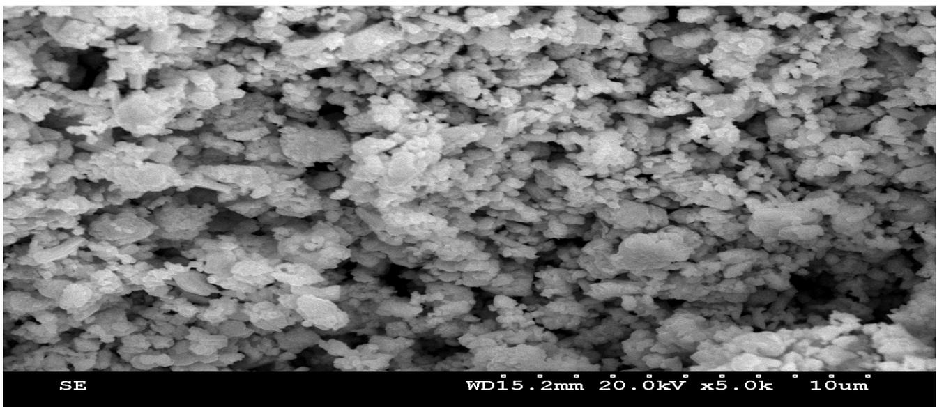
Figure 7: SEM of Dispersed WC at 10  $\mu\text{m}$  Scale and 5,000 Magnification
