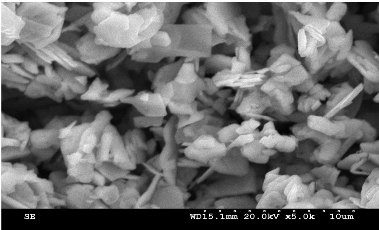
Figure 4: SEM of Dispersed  $\alpha$ -Mo<sub>2</sub>C at 10  $\mu$ m Scale and 5,000 Magnification
