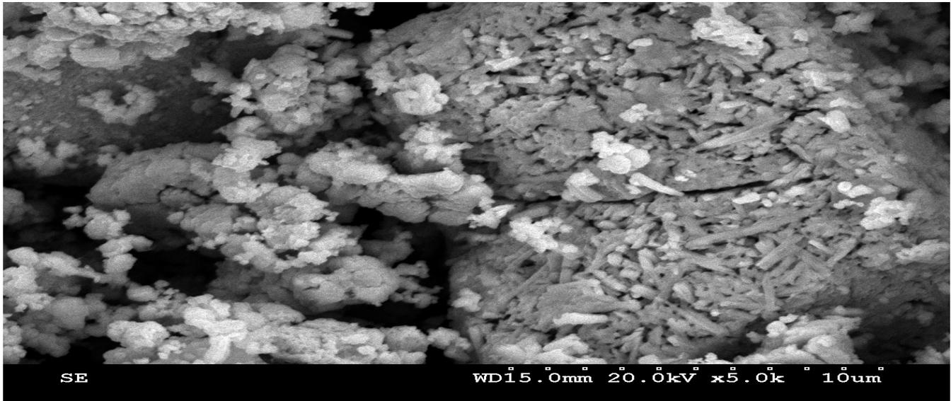
Figure 6: SEM of Undispersed WC at 10  $\mu\text{m}$  Scale and 5,000 Magnification
