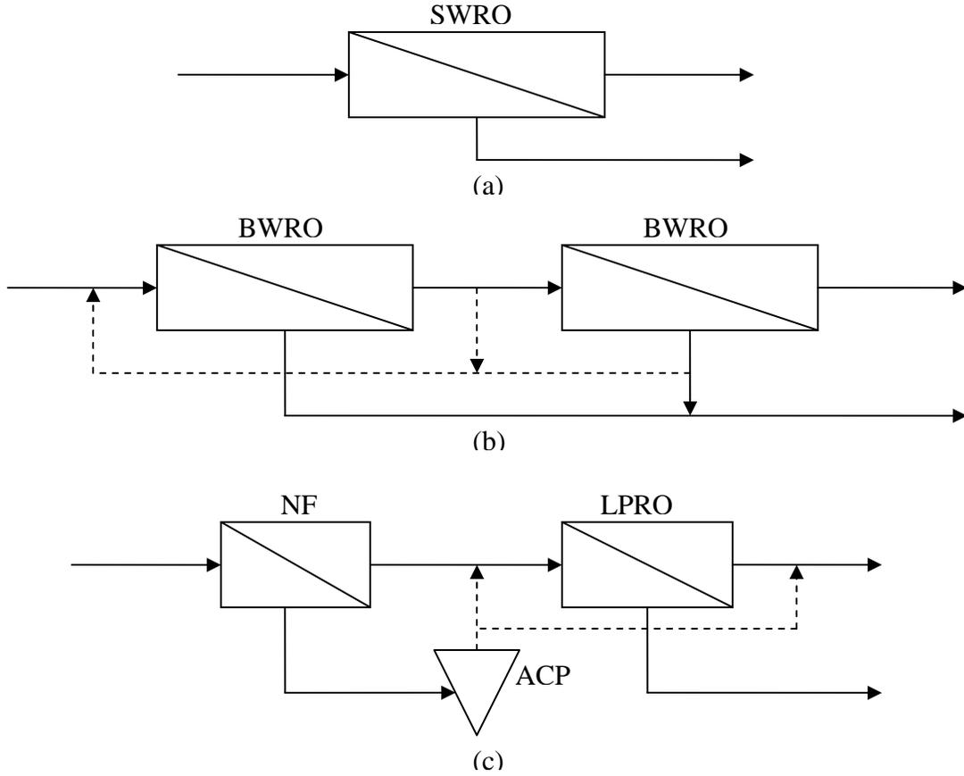
**Figure 1:** (a). Conventional approach using a single pass SWRO. (b). Multi-pass approach using BWRO followed by another BWRO. (c). Multi-pass approach using NF followed by LPRO while incorporating Accelerated Chemical Precipitation (ACP). Dash line represents other alternatives of redirecting flows.
