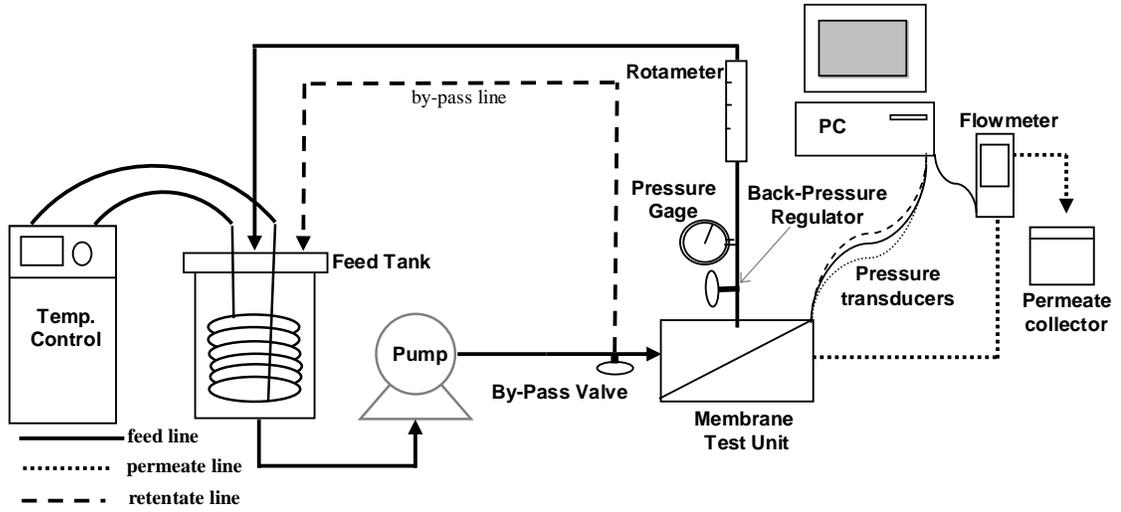
**Figure 2:** Experimental crossflow RO system.
