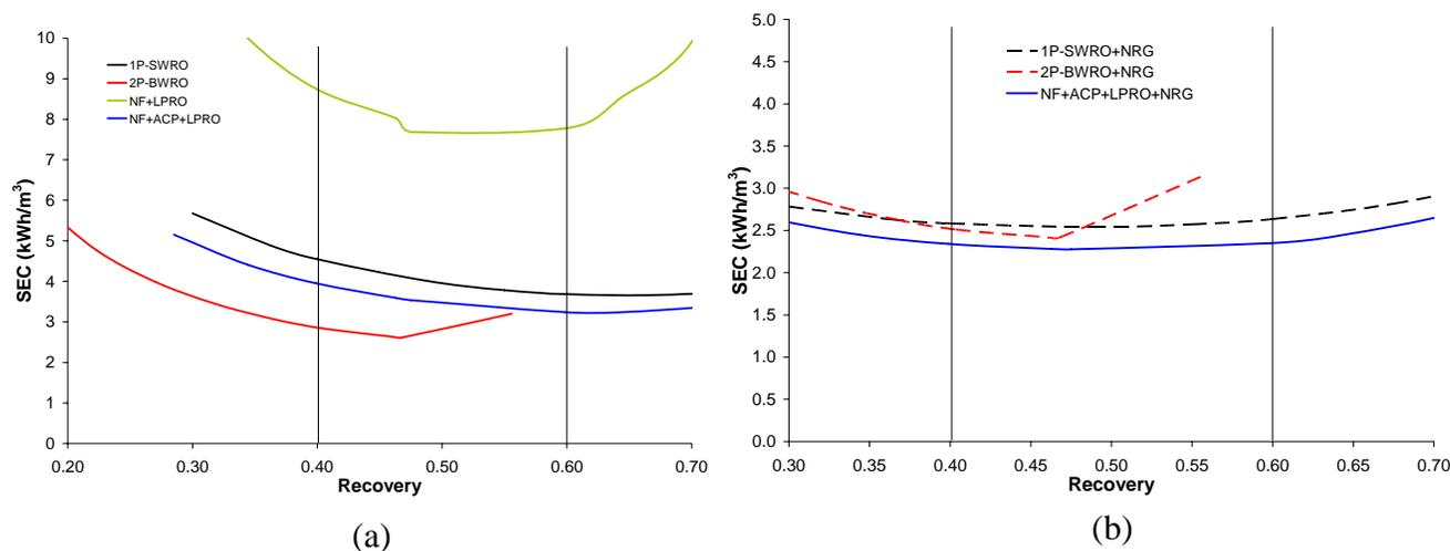
Figure 4: Specific energy consumption for all three system configurations (a) without energy recovery and (b) with energy recovery. Note the use of an inter-stage chemical precipitation process to demineralize stage 1 nanofiltration concentrate and re-blend with permeate substantially reduces the overall energy demand.
