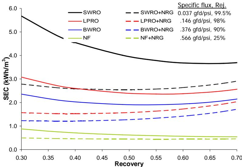
Figure 3: Specific energy consumption (SEC) with and without energy recovery (ER) for each type of membrane treating raw seawater.
