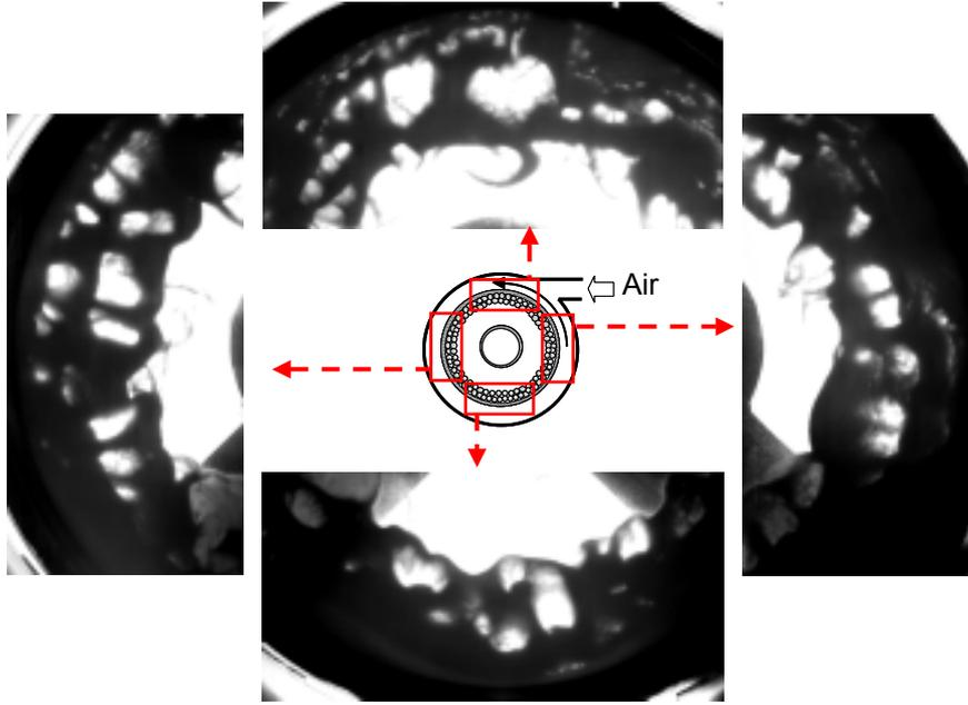
**Figure 4.** Visualized bubbling behavior in RFB.  $G_0=20.0$ ;  $(u-u_{mf})|_{L=0}=0.170$  m/s.
