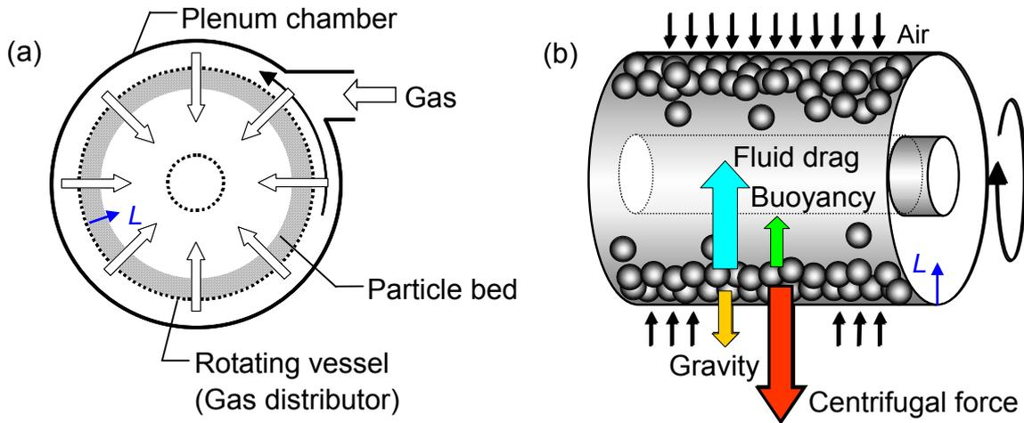
**Figure 1.** Rotating fluidized bed (RFB) system. (a) Front view; (b) side view.
