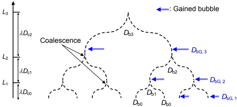
**Figure 2.** Schematic diagram of the proposed bubble growth model in RFB.
