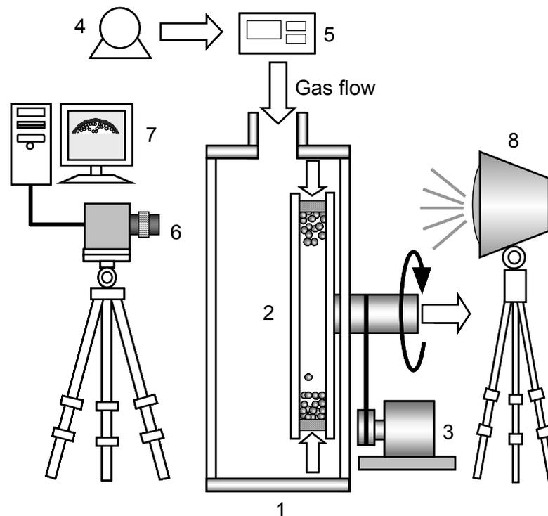
**Figure 3.** Experimental set up. (1) Plenum chamber; (2) rotating vessel (gas distributor; I.D. 250 mm × D. 5 mm); (3) motor; (4) blower; (5) mass flow meter; (6) high-speed video camera; (7) data acquisition system for high-speed video camera; (8) metal halide lamp.
