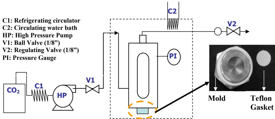
**Figure 1a. Experimental setup for fabrication of micro-porous foams using high pressure CO<sub>2</sub> foaming method**
