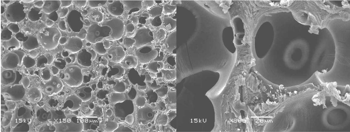
**Figure 2a. Scanning Electron Micrographs of the porous structure of 5% paclitaxel loaded PLGA 5050 foams**
