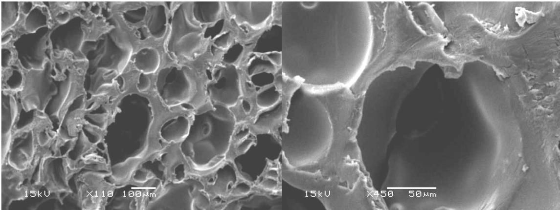
**Figure 2b. Scanning Electron Micrographs of the porous structure of 5% paclitaxel loaded PLGA 8515 foams**
