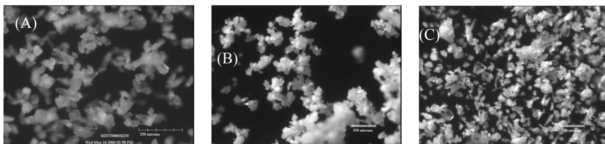
**Figure 3:** Microscopic images of wet granules obtained from different granulators (A) KG-5, 10 $\times$ ; (b) PMA1, 5 $\times$ ; and (C) PMA65, 5 $\times$
