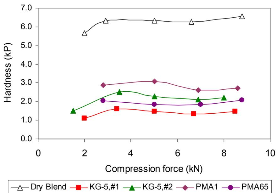
**Figure 5:** The profiles of hardness with compression force.
