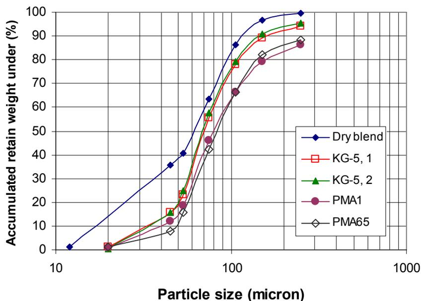
**Figure 4:** Particle size distribution of dry blend and dried granules formed in different granulators.
