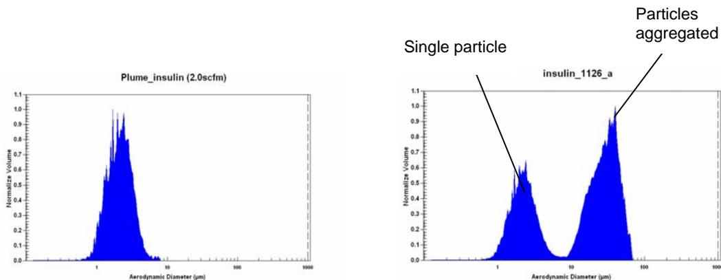
Figure 3 Particle Size Distribution of the Insulin Powder by TSI Particle Size Distribution Analyzer (Left: Gas-solids plume flow out of the dispenser; Right: Bulk powder )
