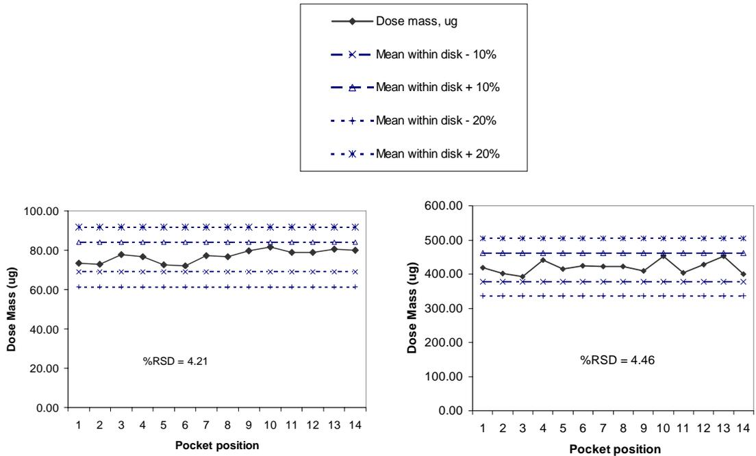
Figure 4 Uniformity test for dispensing device using spray dried insulin powder (2.10µm) within different size disks
