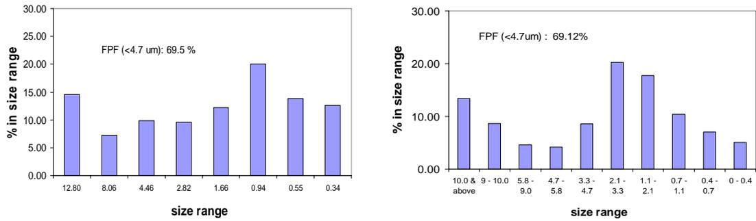
Figure 5 Aerodynamic particle size distribution of spray dried insulin powder (2.10µm) delivered via new DPI Using Andersen cascade impactor (left) and Next Generation Impactor (right)
