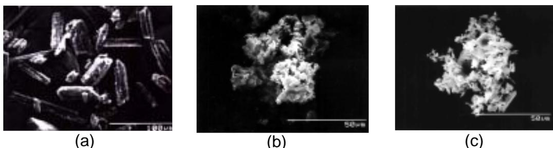
**Figure 3.** SEM photographs of granules. (a) Original, (b) FG-SCF (10 MPa, 343 K), (c) FG-SCF (10 MPa, 343 K) with D-mannitol.
