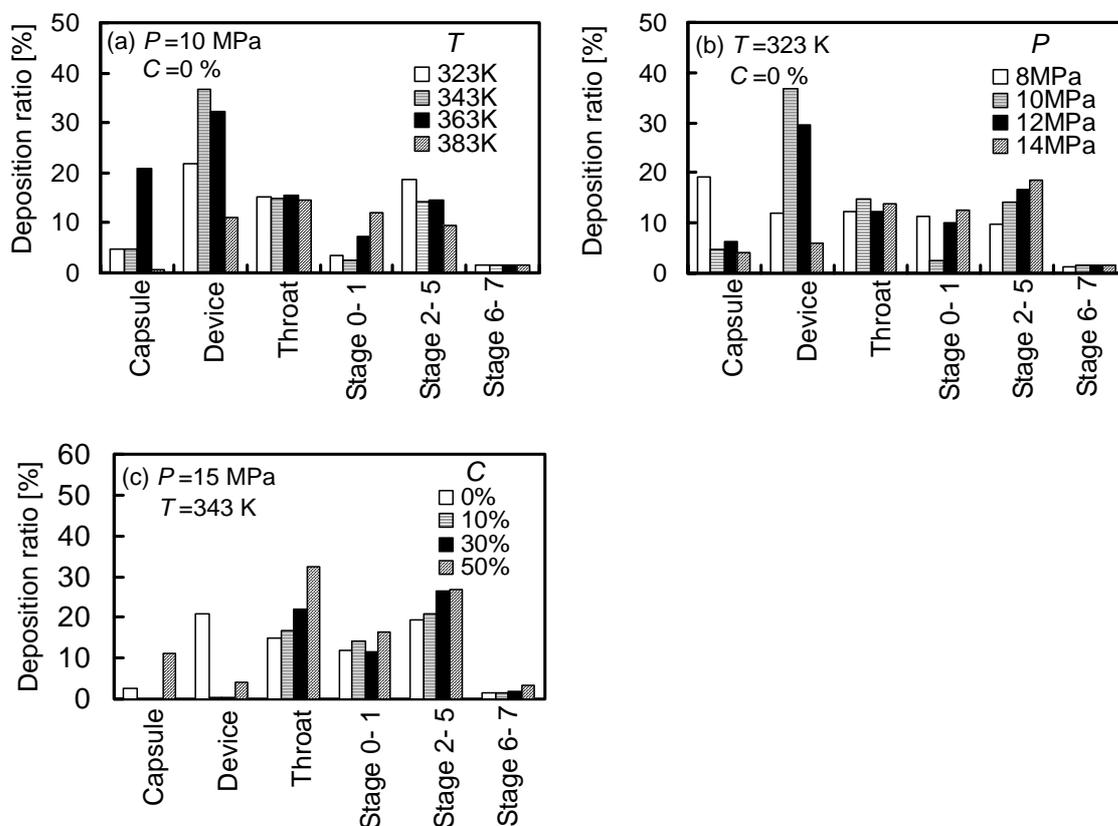
**Figure 7.** The effect of operating parameters on deposition ratio. (a)  $P=15$  MPa,  $C=0\%$ , (b)  $T=343$  K,  $C=0\%$ , (c)  $P=15$  MPa,  $T=343$  K.
