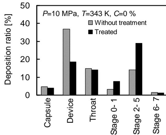
**Figure 8.** The effect of electrostatic treatment on deposition ratio.
