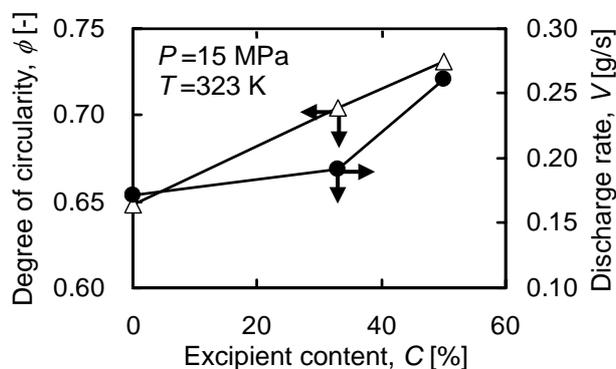
**Figure 6.** Change in degree of circularity and discharge rate with excipient content ( $P=15$  MPa,  $T=323$  K).
