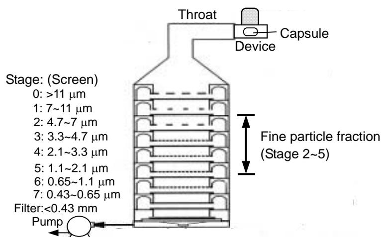
**Figure 2.** Schematic diagram of cascade impactor.
