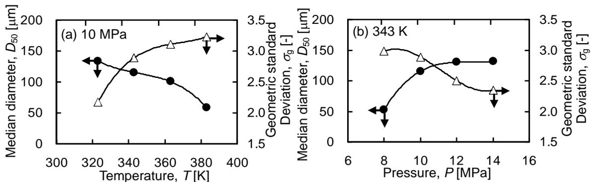
**Figure 4.** The effect of temperature and pressure on median diameter and geometric standard deviation (without excipient). (a)  $P=10$  MPa, (b)  $T=343$  K.
