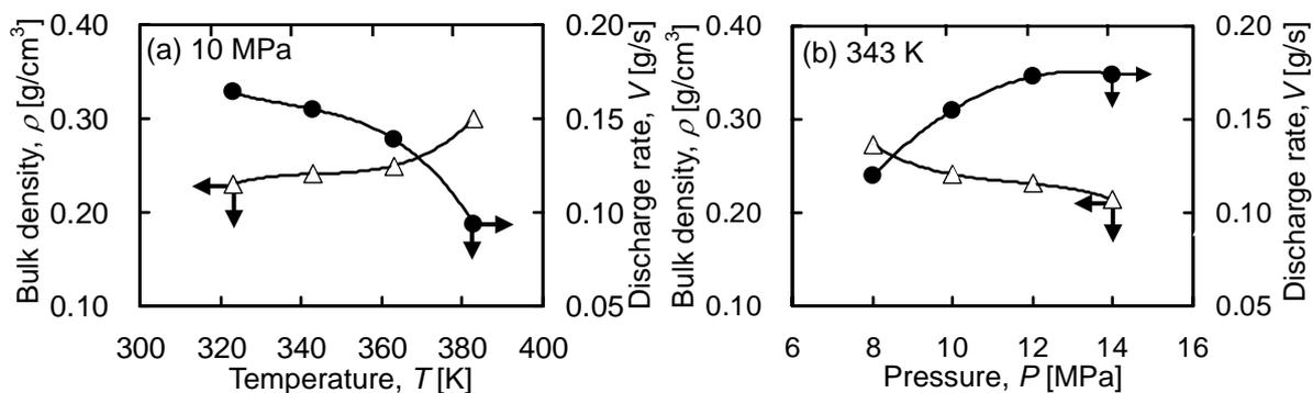
**Figure 5.** The effect of temperature and pressure on bulk density and discharge rate (without excipient) (a)  $P=10$  MPa, (b)  $T=343$  K.
