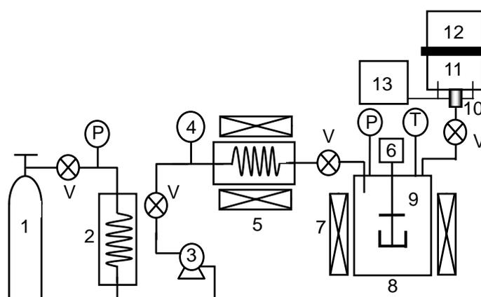
**Figure 1.** Schematic diagram of experimental set-up. (1) CO<sub>2</sub> cylinder, (2) Cooler, (3) Pump, (4) Flowmeter, (5) Pre-heater, (6) Motor, (7) Heater, (8) Vessel, (9) Paddle, (10) Nozzle, (11) Vessel, (12) Particle collector, (13) Hot air generator, P : Pressure gauge, V : Valve, T : Thermometer.
