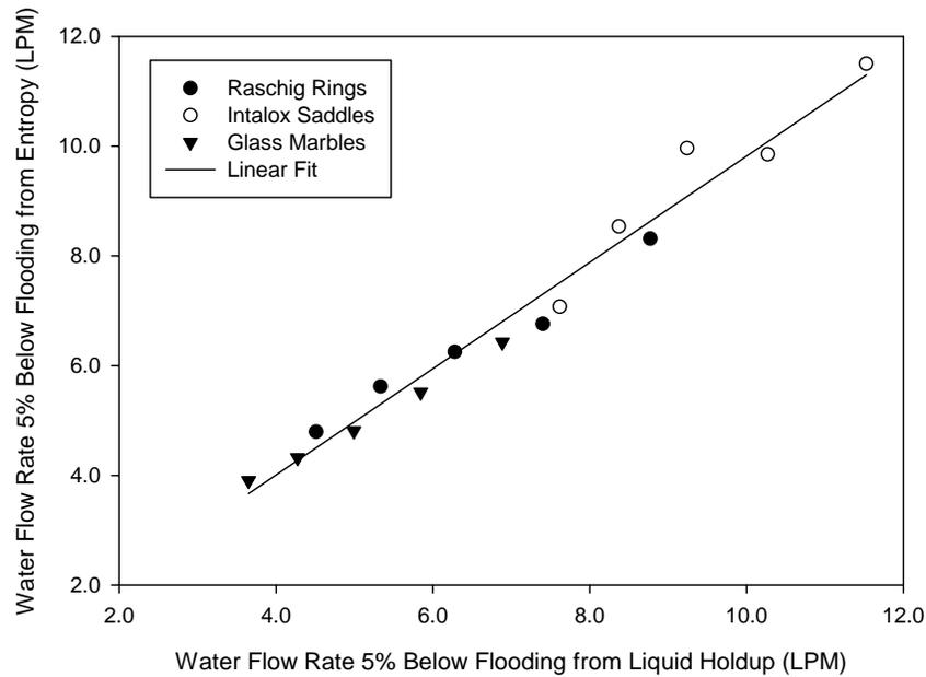
**Figure 10: Correlation between critical water flow rates obtained from the entropy of the microphone signal and liquid holdup**
