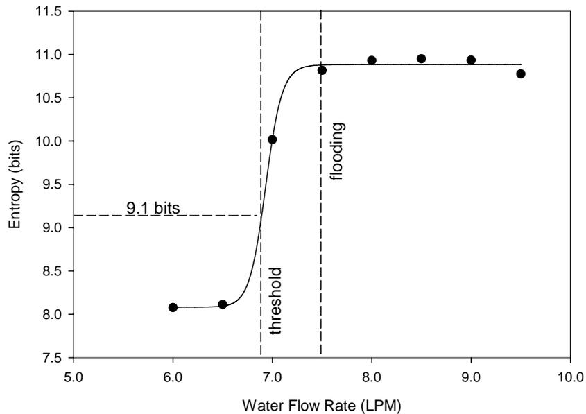
**Figure 9: Entropy versus water flow rate at 50 LPM with Raschig ring packing and a threshold**
