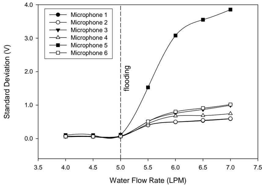
**Figure 3: Standard deviation versus water flow rate at 70 LPM air flow with Raschig ring packing**
