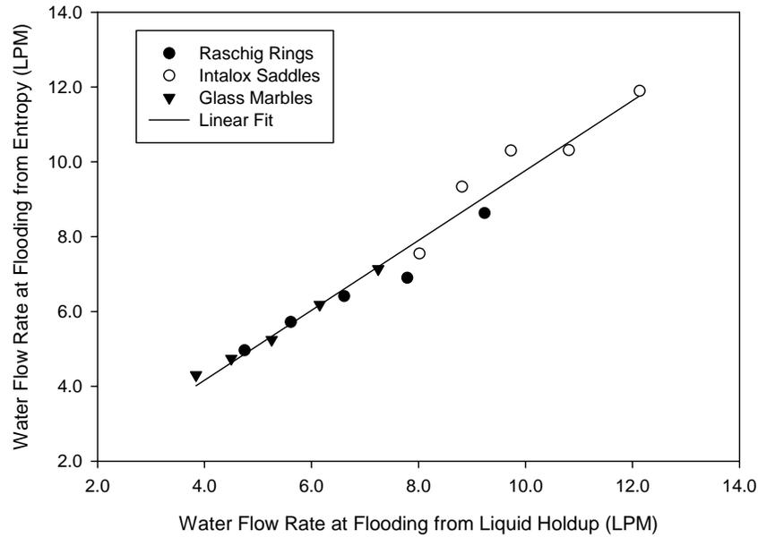
**Figure 7: Correlation between flooding water flow rates obtained from the entropy of the microphone signal and the liquid holdup**
