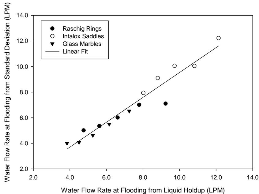
**Figure 5: Correlation between flooding water flow rates obtained from the standard deviation of the microphone signal and the liquid holdup**
