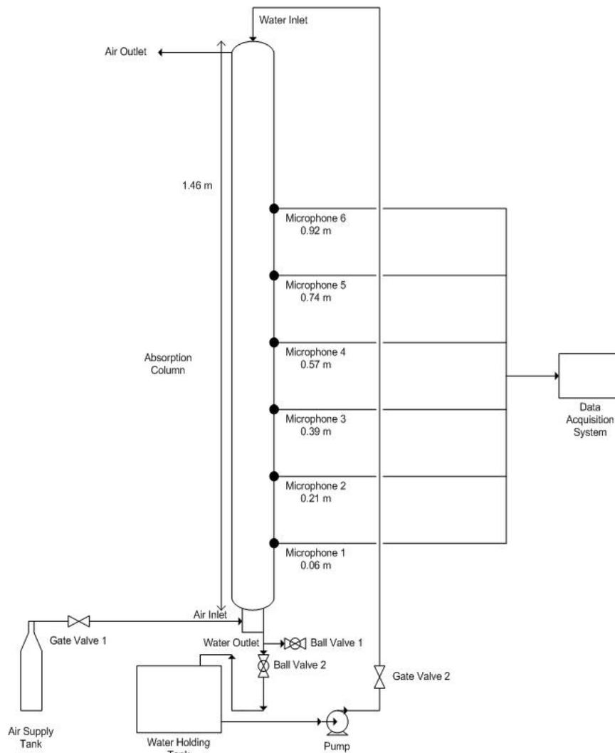
**Figure 1: Experimental apparatus**
