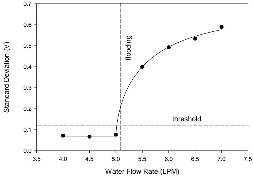
**Figure 4: Threshold for standard deviation versus water flow rate at 70 LPM air flow with Raschig ring packing**
