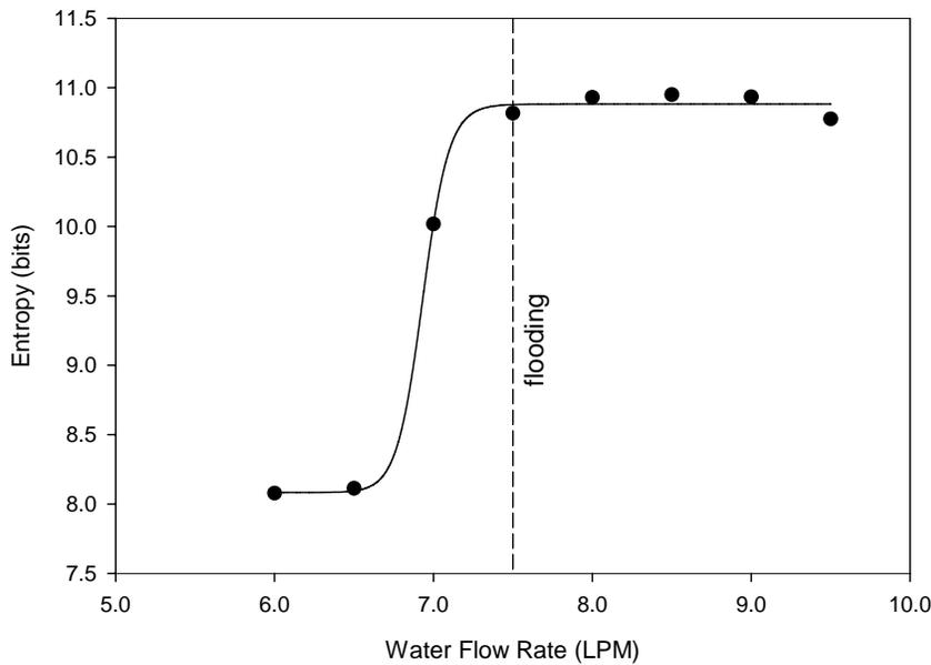
**Figure 6: Correlation between flooding water flow rates obtained from the standard deviation of the microphone signal and the liquid holdup**
