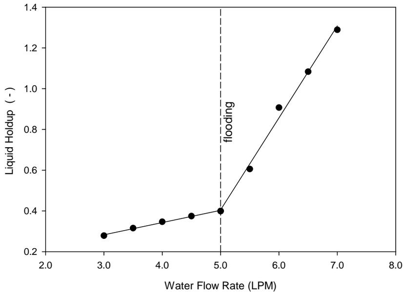
**Figure 2: Liquid holdup versus water flow rate at 70 LPM air flow with Raschig ring packing**
