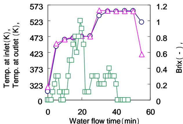
Fig.6 Changes in temperature of HCW and brix of effluent for two-step heating treatment of wheat straw
