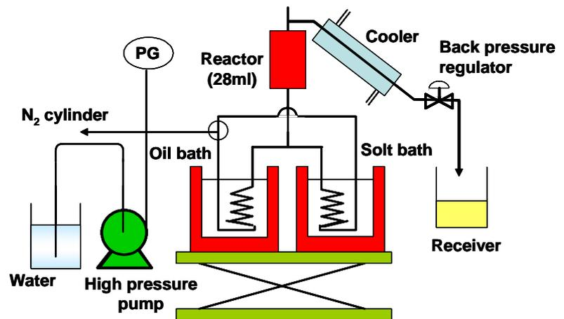
Fig.1 Schematic diagram of Type-1 HCW-flow reactor
