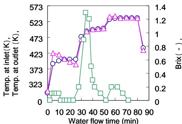
Fig.8 Changes in temperature of HCW and brix of effluent for three-step heating treatment of wheat straw
