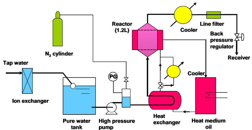
Fig.2 Schematic diagram of Type-2 HCW-flow reactor
