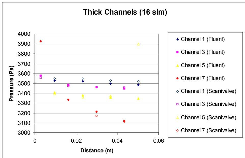
**Figure 4.** Comparison between pressure transducer array and CFD results.
