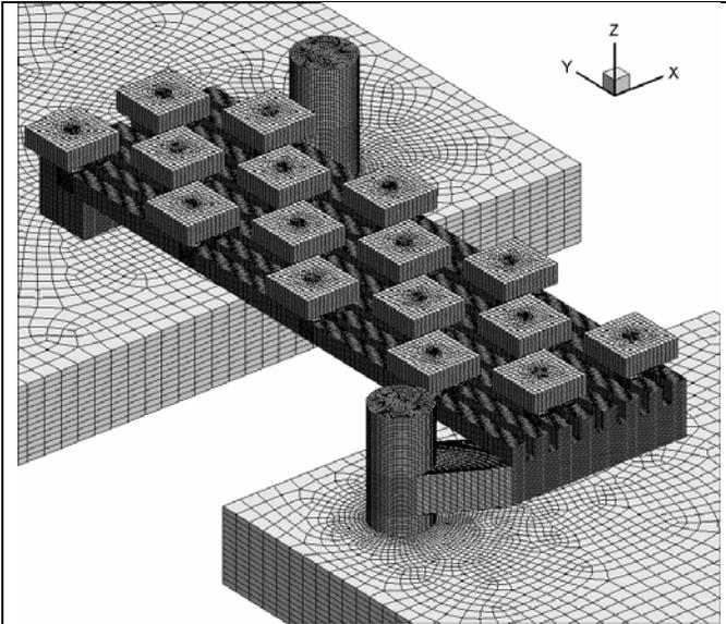
**Figure 2.** Heat exchanger mesh.
