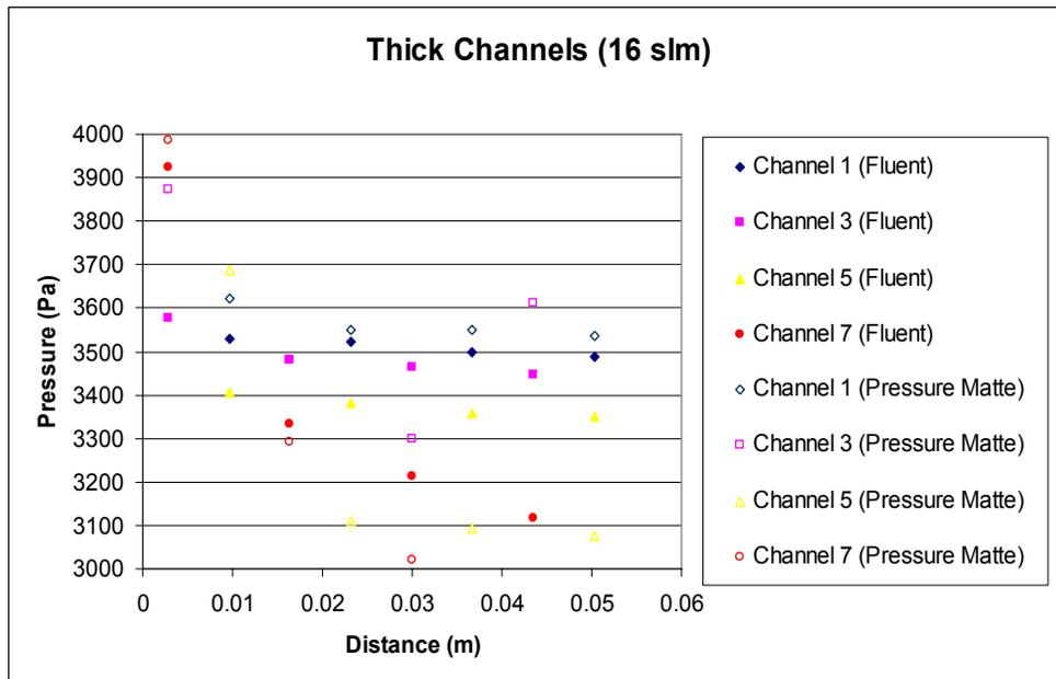
**Figure 7.** Comparison between pressure mat and CFD results.
