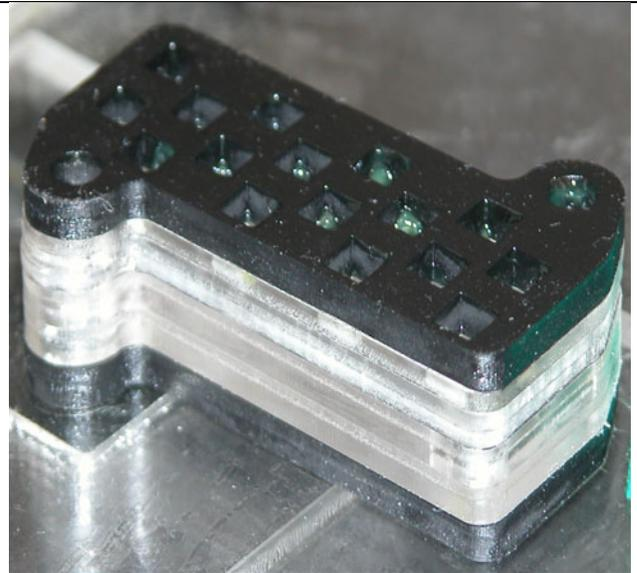
**Figure 3.** Plexiglas part with conformal top and bottom layers.
