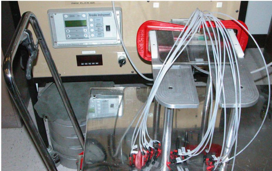
**Figure 1.** Array of tubes used to determine pressure drop across heat exchanger.
