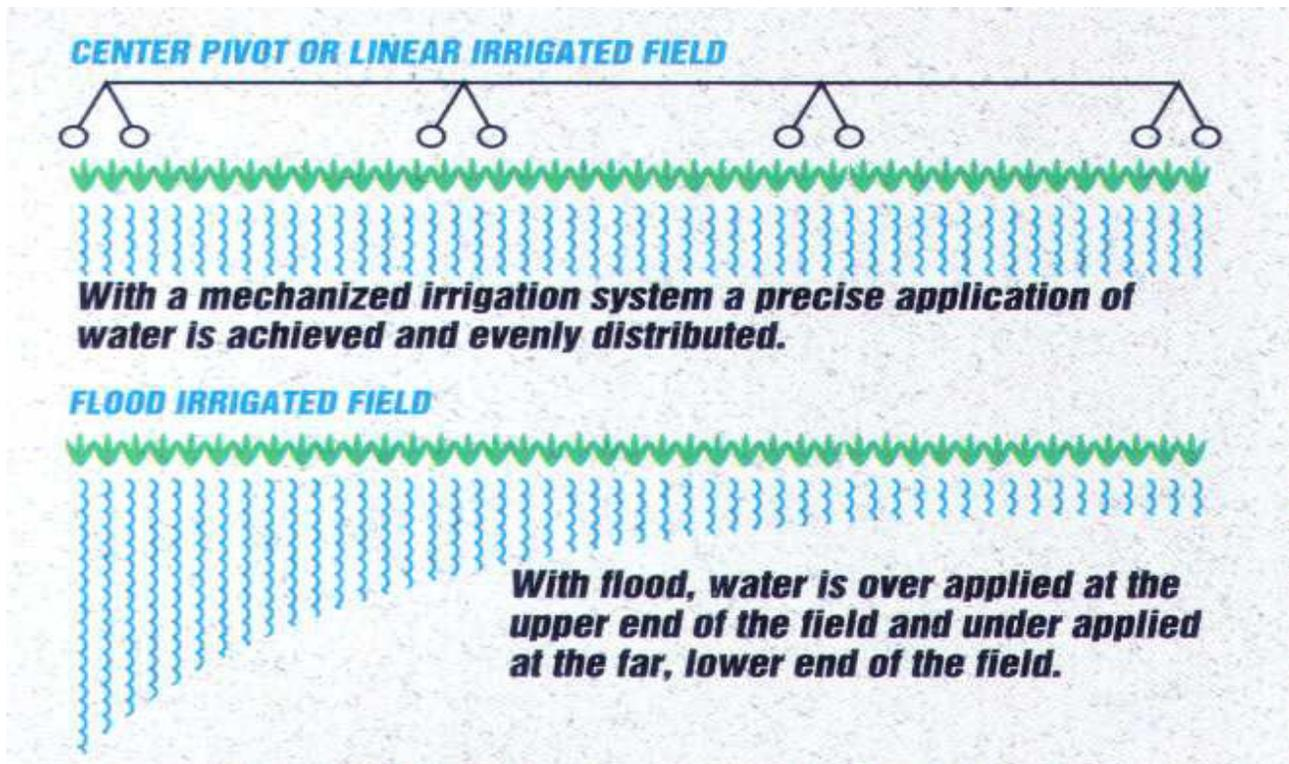
Figure 2. Irrigation Application Comparison (courtesy Valmont Industries, Inc.)
