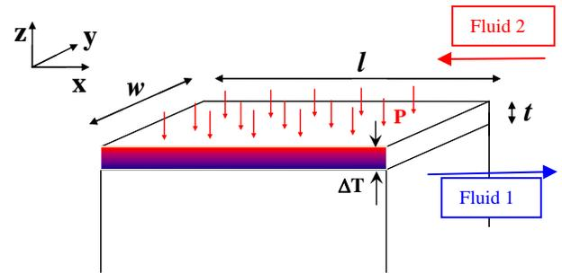
Figure 5. Loading Conditions for Thermo-Mechanical Stresses in Heat Exchanger Plate
