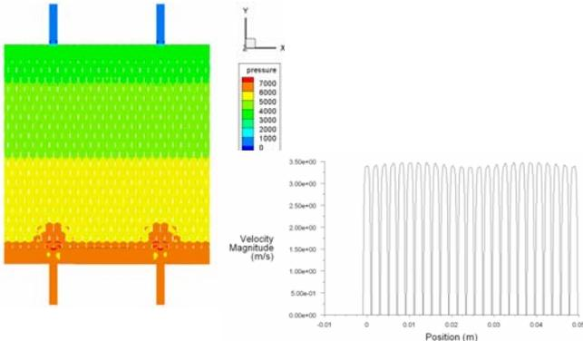
Figure 7b. Optimized Plate Design and its Associated Flow Distribution
