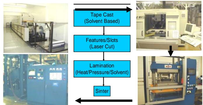
Figure 8. LOM Method for Ceramic Planar Structures
