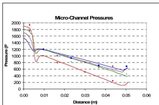
Figure 10. A Comparison: CFD vs Experimental Results.
