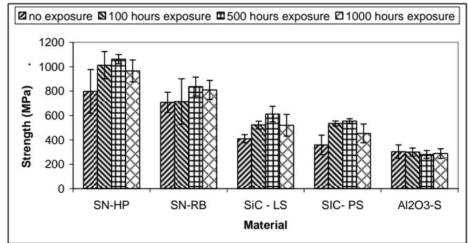
Figure 4b. Strength Change for 1000 hr Exposure Samples
