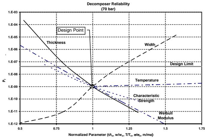
Figure 6. Probability of Failure for Heat Exchanger Plate
