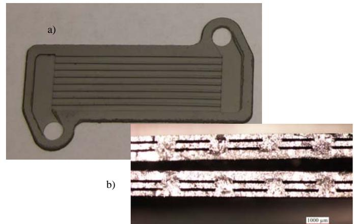
Figure 9. Sub-scale Heat Exchanger Plates – a) Uncapped Plan view [Channels (LxWxD): 45mm x 1250 $\mu$  x 250 $\mu$ .], b) Fractured Cross-Section of 2 Plates.
