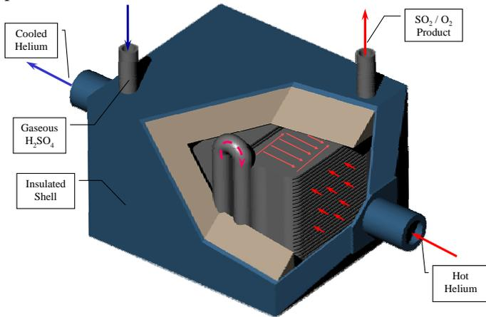
Figure 2. Shell and Plate Design of a Compact Heat Exchanger
