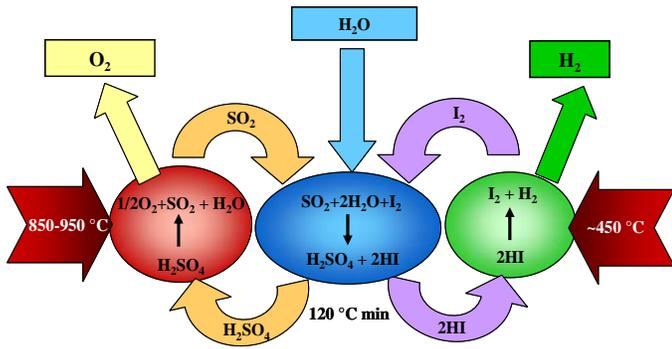
Figure 1. Simplified Sulfur Iodine Cycle
