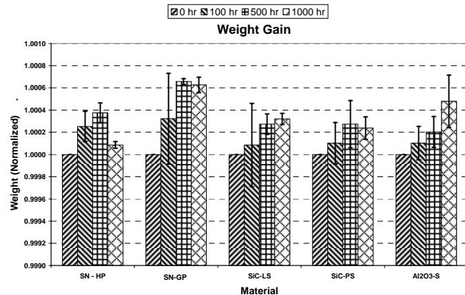
Figure 4a. Weight Gains for 1000 hr Exposure Samples
