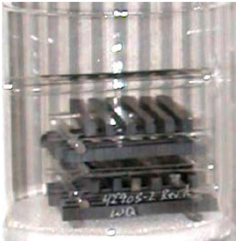
**Figure 3. Bend bar arrangement in small sample cups.**
