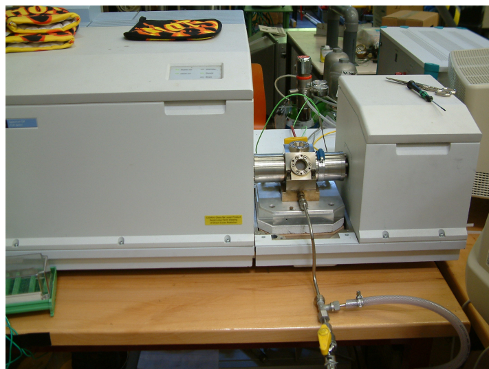
Figure 2: Heated grid reactor in FT-IR compartment
