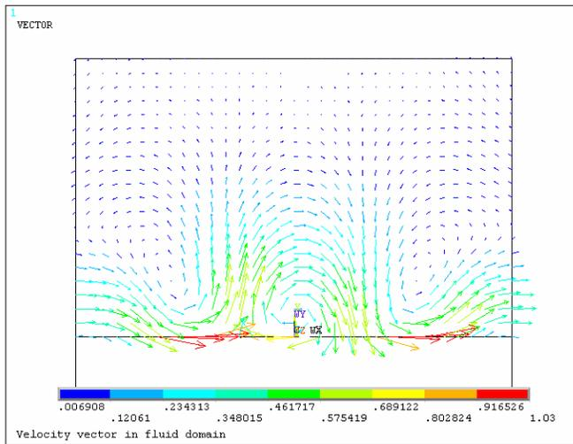
**Figure 5. Velocity vector plot showing fluid recirculation over the IDT region.**
