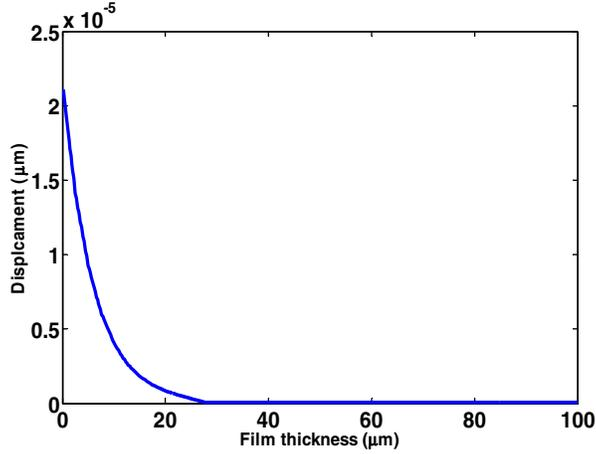
**Figure 3. Displacement profile along the film thickness induced as a result of leakage of ultrasonic SAW power into the fluid. The exponential decay with distance from the source is similar to that of Leaky SAW.**
