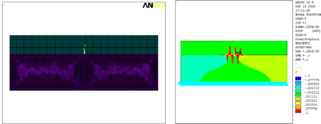
**Figure 1. (a) Finite element model of liquid loading on a SAW device. (b) Contour plot showing the direction of movement of IDT fingers located at the center on the surface of the piezoelectric device at  $t=2.5$  ns.**
