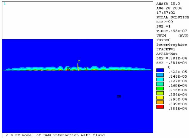
**Figure 4. Displacement contours in fluid region for an applied AC peak voltage of 1 V. The wave decays with distance from the IDT fingers located at the center of the device. The displacements in the solid have been suppressed for clarity.**
