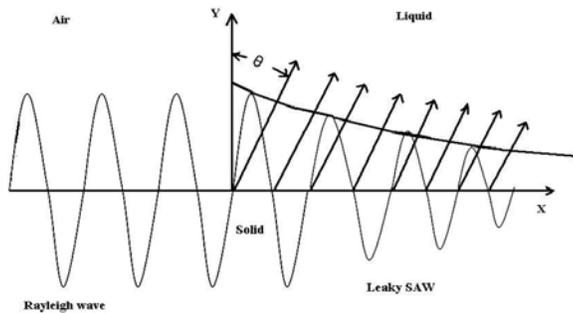
**Figure 2. Ultrasonic radiation into the fluid medium.**
