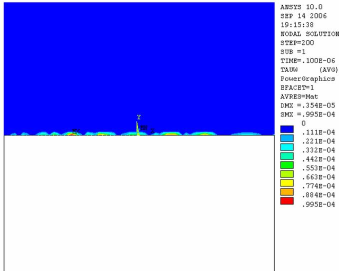
**Figure 6. Shear stresses (MPa) generated as a result of the recirculation at the surface of the SAW device. The applied input voltage was 0.1 V and the fluid viscosity was 10 cP.**
