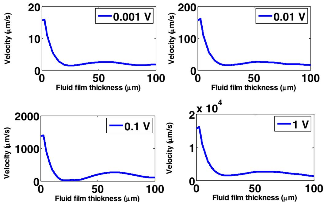
**Figure 7. Simulated streaming velocity profiles along the thickness of the fluid film. The applied input voltage was varied from 1 mV to 1 V. The streaming velocity varies approximately linearly with the applied input voltage.**
