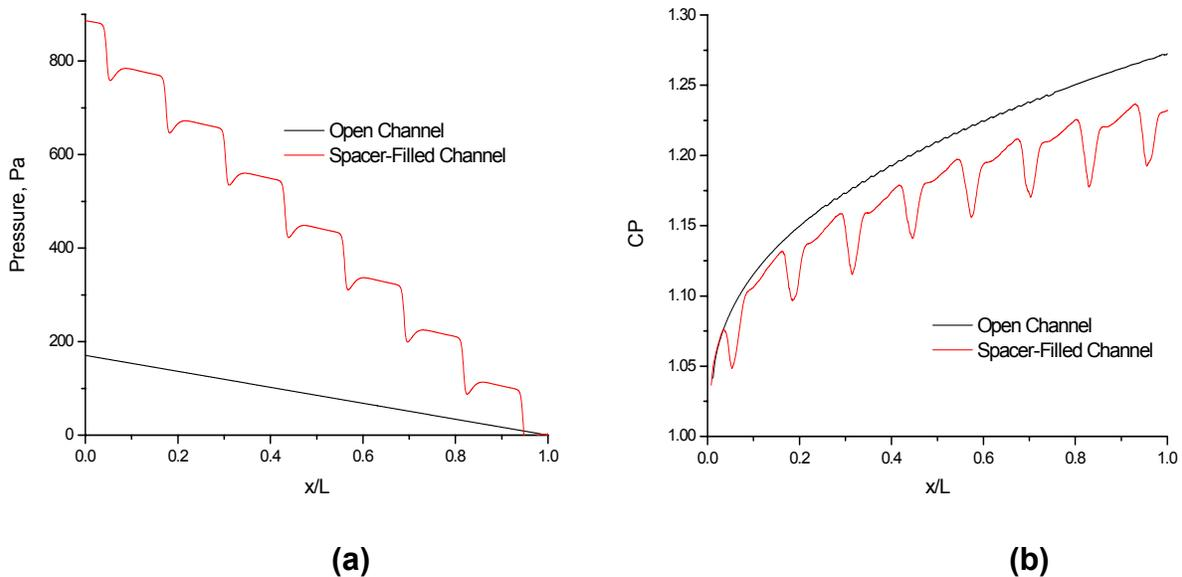
**Figure 1.** Comparison of (a) axial pressure losses and (b) concentration polarization in open and spacer-filled channels.
