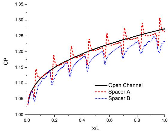
**Figure 2.** Evidence of spacer-induced stagnation zones as shown by Spacer A. Spacer B shows a consistent reduction of CP.
