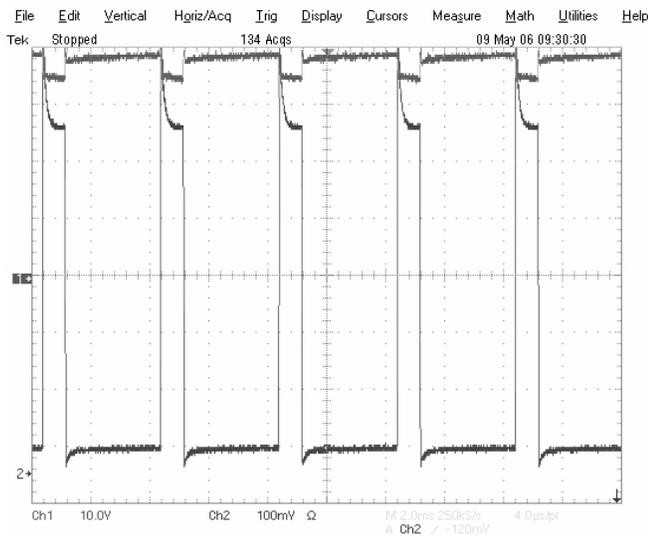
**Figure 3.** Two Nexa™ stacks (#881 and #515) operated in parallel and pulse tested at a total current (bottom line) of 60 A and pulse voltage (top line) between 35.4 V and 39.4 V at 250 Hz frequency and 20% duty cycle. Before tests at 60 A, Nexa™ stack #881:  $T_s=54.5^\circ\text{C}$ ,  $E_s=31.36\text{ V}$ ,  $I_s=29.45\text{ A}$ ,  $P_s=925\text{ W}$ ; Stack #515:  $T_s=60.6^\circ\text{C}$ ,  $E_s=31.66\text{ V}$ ,  $I_s=36.47\text{ A}$ ,  $P_s=1155\text{ W}$ .
