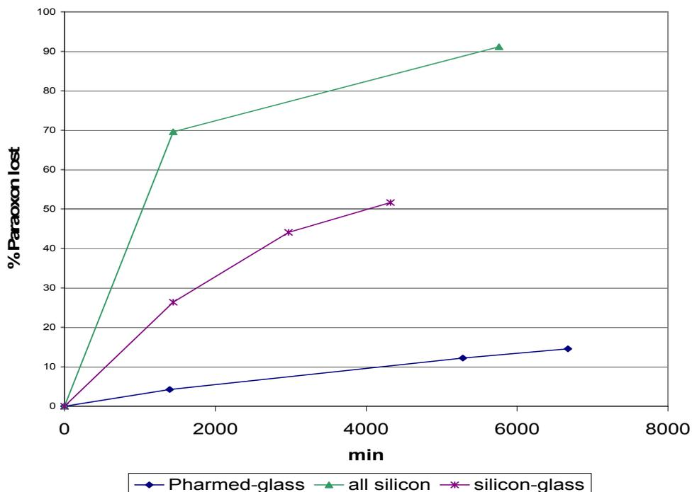
**Figure 3.** Comparison of paraoxon loss with different tubing (no enzyme, 50 ml, sterile circulating loop system).
