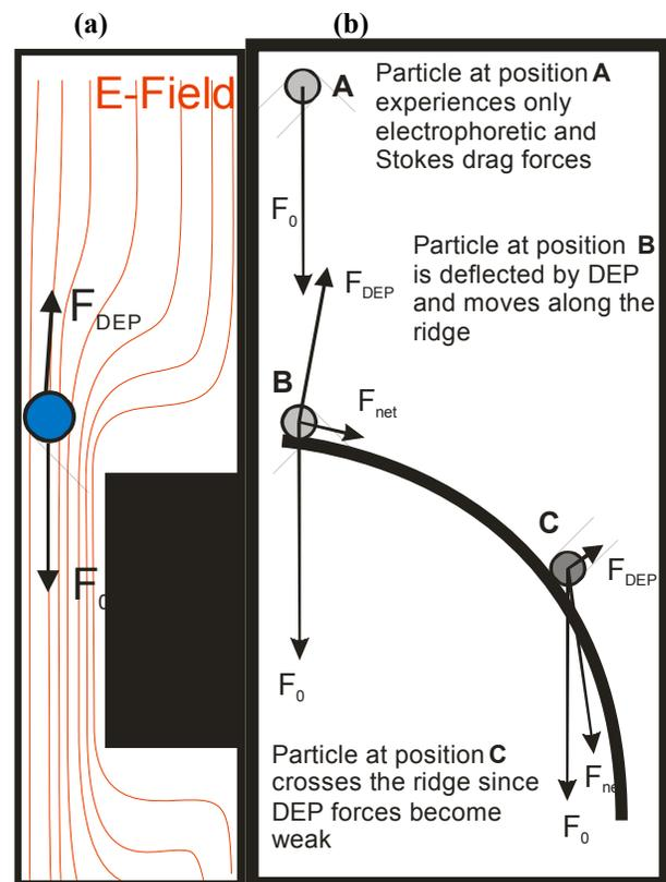
Figure 2. (a) Side view of ridge, showing constriction and attendant increase in local electric field.  $F_0$ : motive force on particle in absence of DEP.  $F_{DEP}$ : DEP force away from high electric field region. (b) Top view of microdevice, showing forces on a particle as it approaches and moves
