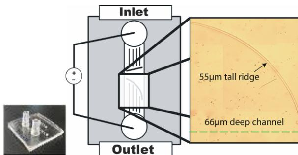
Figure 1. Overview of microdevice. Left: picture of device. Middle: schematic of device with location of electrodes. Right: blowup of region with curvilinear ridge.
