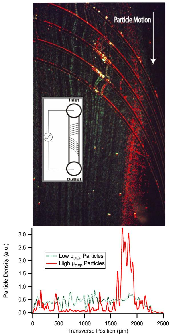
Figure 4. Particles sorted by DEP mobility. Fluorescence micrograph (top) shows deflection of particles with high DEP mobility along the curvilinear ridges (18V/cm DC + 600V/cm AC). The inset diagram illustrates the redundant ridge layout. Time averaged particle density scans (low pass filtered) show the deflection dependence on dielectrophoretic mobility.
