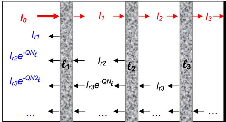
Figure 1 - Model of Reflected Light Intensity Measurement
