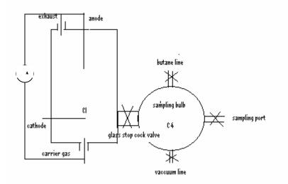
It is a 3cm\*10cm circular tube made of pyrex glass. It houses mainly an anode and a cathode. The anode is a stainless steel (100 mesh) plate. The cathode is a 2.5 cm long tube of internal diameter 1.5mm. It has 2 holes and a few projected thorns along the sides.
