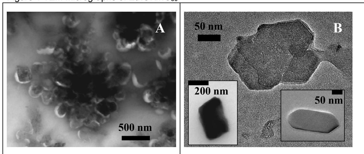
Figure 2 TEM micrographs of aqu/ $nC_{60}$  --2 weeks mixing
