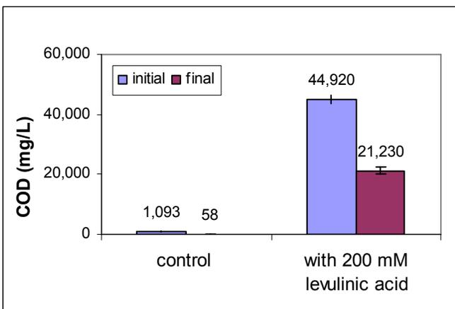
Figure 3: The Chemical oxygen Demand (COD) of the acetic acid media, with and without the inhibitor.
