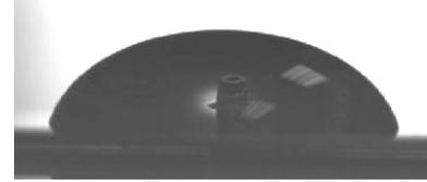
□ Fluorine plasma (CHF<sub>3</sub>) treated PMMA surface  $\theta \sim 108^\circ$
