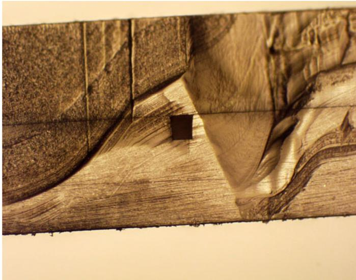
CO<sub>2</sub> bonding (200psi, 75psi, 1 hour, PLGA interlayer)
