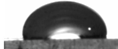
□ Fluorine plasma treated micro-patterned PMMA surface  $\theta > 160^\circ$ ,  $f=0.1$
