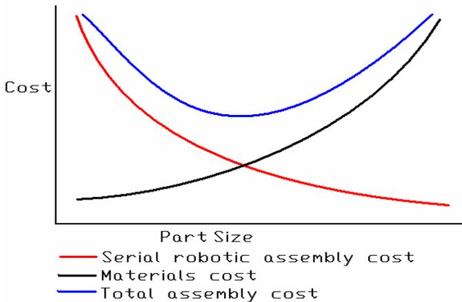
Figure 1: The blue curve represents the total cost of assembly using pick and place robots, whereas the red and black curves are the cost of operating serial assembly robots and the cost of materials, respectively.
