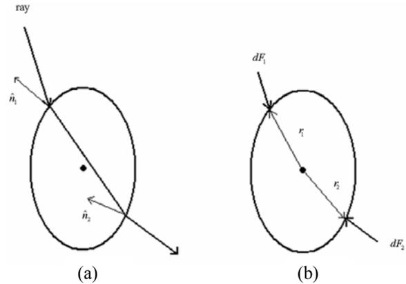
Figure 3: A ray tracing diagram (a) is shown for a single ray propagating through a prolate spheroid with normal vectors  $\hat{n}_1$  and  $\hat{n}_2$ . The free body diagram (b) for such system is shown with differential force contributions  $dF_1$  and  $dF_2$  and moment arms  $r_1$  and  $r_2$ .
