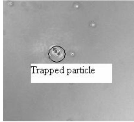
Figure 2: A polystyrene latex microsphere (0.7um diameter) is trapped in an optical tweezers. Astigmatic aberration is visible due to the broadband light used to create the image. Such aberration is not present during the actual experiment. The aberration presented in the image is to show the particle is scattering the incident laser.
