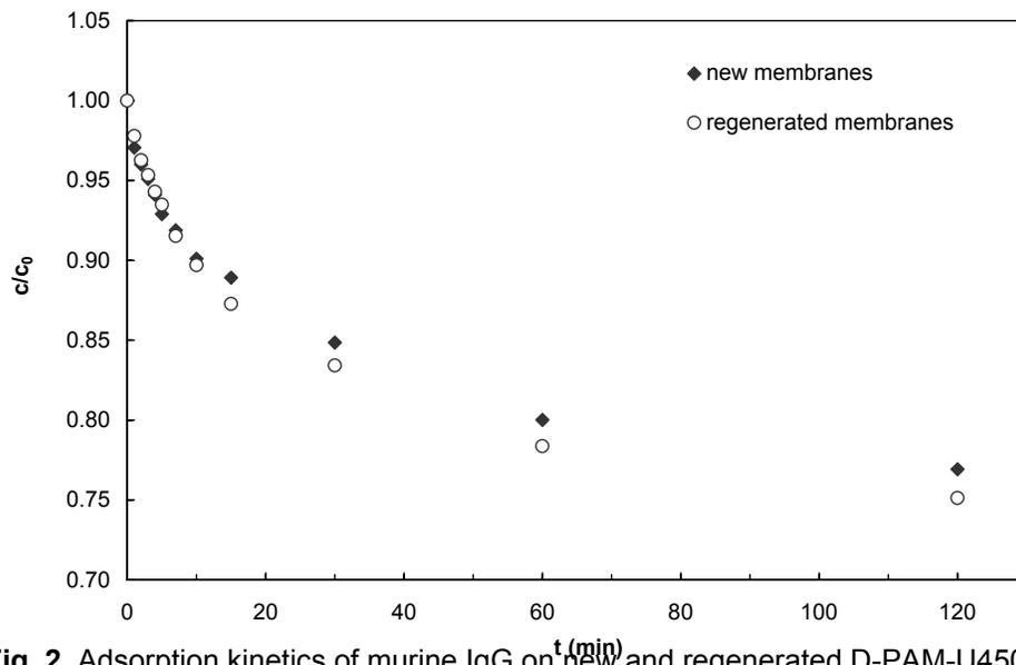
**Fig. 2** Adsorption kinetics of murine IgG on new and regenerated D-PAM-U450 affinity membranes.
