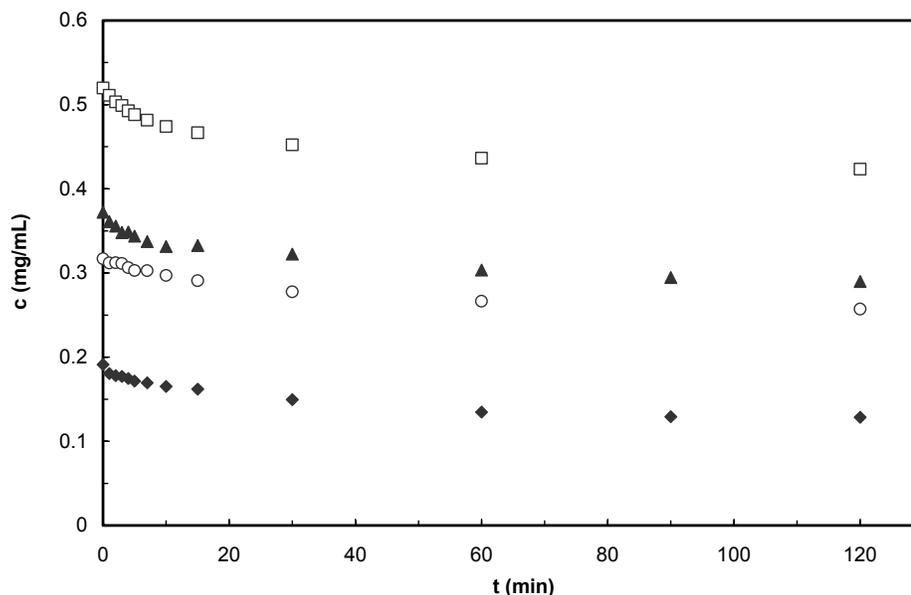
Fig. 1. Adsorption kinetics of murine IgG solutions on D-PAM-U450 affinity membranes.
