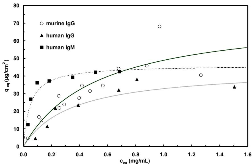
**Fig.3:** Adsorption isotherms of murine IgG, human IgG and human IgM onto D-PAM-U450 affinity membranes.
