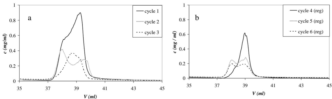
**Figure 3.** Elution step for six subsequent breakthrough curves of IgG on A2P Sartopoxy membranes at 1 ml/min and 0.5 mg/ml: (a) before regeneration; (b) after regeneration.
