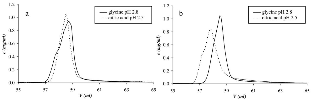
**Figure 6.** Comparison of different elution buffers. Elution step of 1st cycle at 1 ml/min (a), 0.5 ml/min (b) and feed concentration of 0.25 mg/ml.
