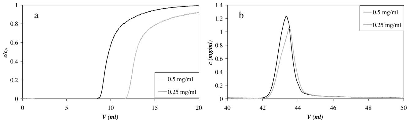
**Figure 5.** Comparison of the 1<sup>st</sup> cycle at 0.5 ml/min and different feed concentration: (a) adsorption step; (b) elution step.
