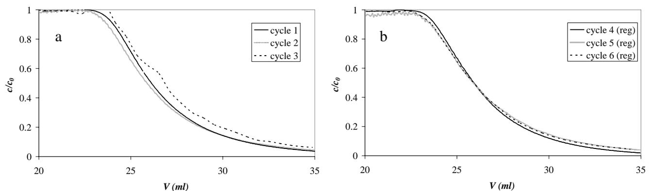
**Figure 2.** Washing step for six subsequent breakthrough curves of IgG on A2P Sartopoxy membranes at 1 ml/min and 0.5 mg/ml: (a) before regeneration; (b) after regeneration.
