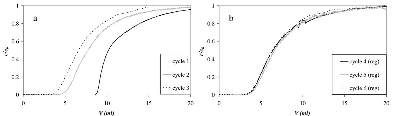
**Figure 1.** Loading step for six subsequent breakthrough curves of IgG on A2P Sartopoxy membranes at 1 ml/min and 0.5 mg/ml: (a) before regeneration; (b) after regeneration.
