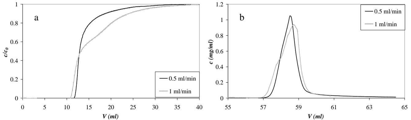
**Figure 4.** Comparison of the 1<sup>st</sup> cycle at 0.25 mg/ml and different flow rates: (a) adsorption step; (b) elution step.
