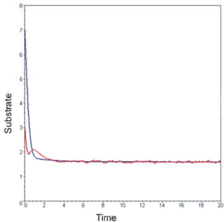
Fig. 8: True and estimated substrate concentration in the presence of white noise of standard deviation 0.2, for truncation order  $N=5$ .
