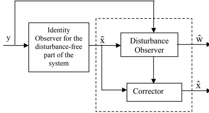
Figure 2: Structure of the modular observer (19) – (21).
