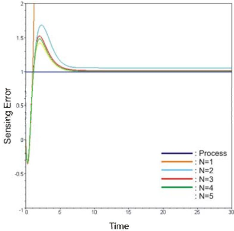
Fig. 12: True and estimated sensing error for different truncation orders.
