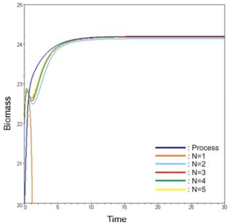
Fig. 10: True and estimated biomass concentration for different truncation orders.
