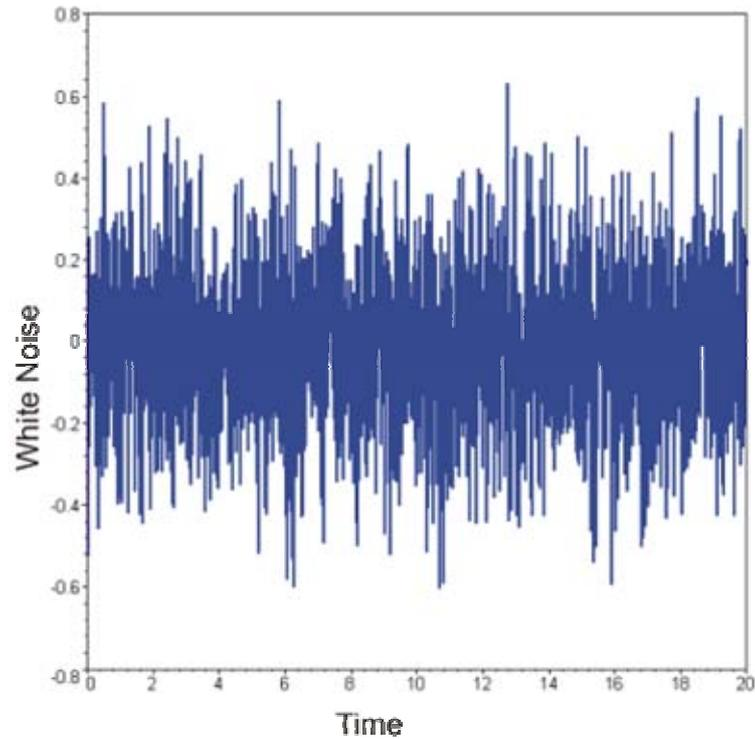
Fig. 6: Simulated white noise of standard deviation 0.2.
