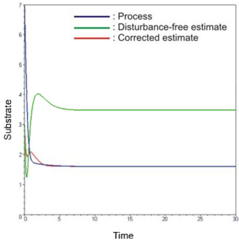
Fig. 4: Disturbance-free and corrected substrate concentration estimates, for truncation order  $N=5$ .
