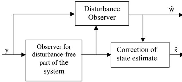
Fig. 1. Modular observer for state and disturbance estimation
