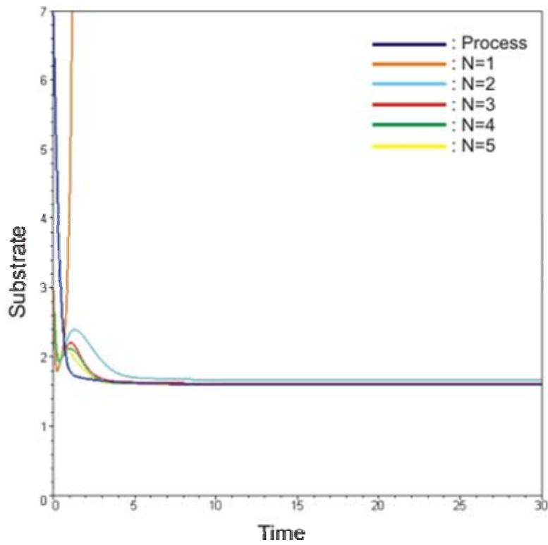
Fig. 11: True and estimated substrate concentration for different truncation orders.
