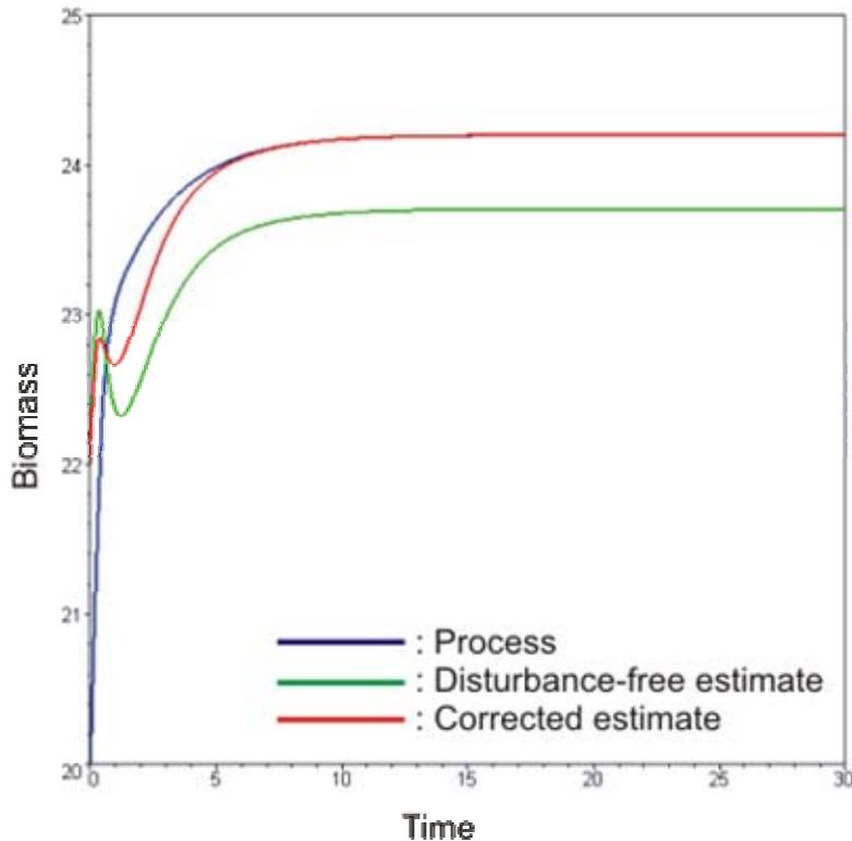
Fig. 3: Disturbance-free and corrected biomass concentration estimates, for truncation order  $N=5$ .
