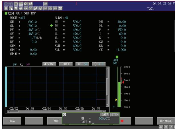
Fig. 10 Tuning panel to modify alarm limits
