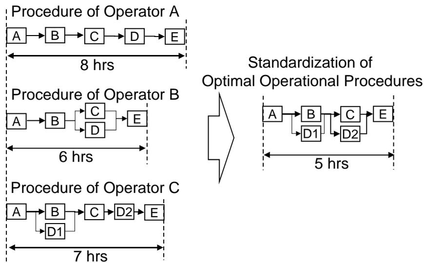
**Fig.5** Standardization of Optimal Operational Procedures
