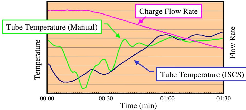
**Fig.8** Application for Decomposition Furnace Decoking Operation
