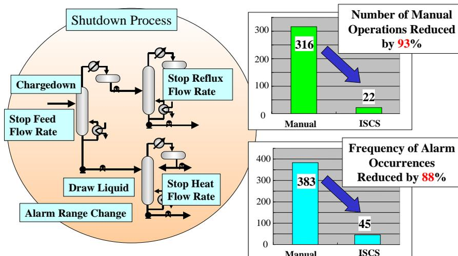
**Fig.6** Application for Distillation Column Shutdown Operation
