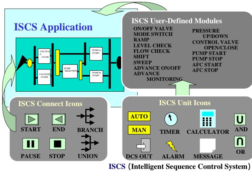
**Fig.3** ISCS Standard Module
