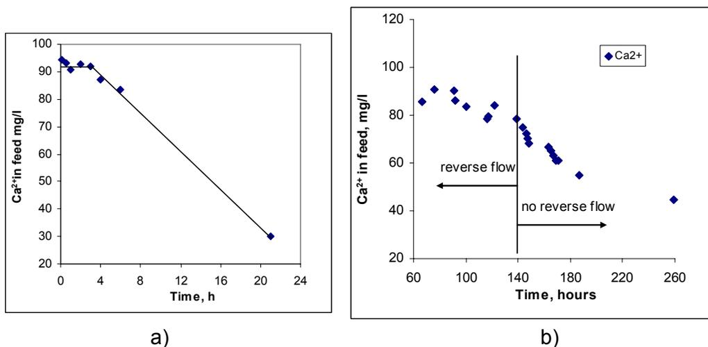
**Figure 4:** Pilot RO runs on feed solution slightly undersaturated with respect to CaCO<sub>3</sub> (LSI = -0.04) and 70% recovery (concentrate LSI = 1.51) . a) without flow reversal b) with flow reversal
