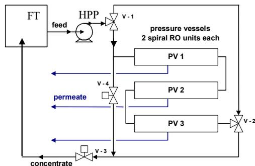
**Figure 1:** Pilot flow reversal scheme. In forward flow, valves v-1 and v-2 are in up position and valve v-4 is closed. In reverse flow these valves are in the opposite position.
