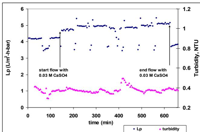
Figure 3: Switch experiment, Run conditions as in Figure 2, every 60 minutes, solution of 0.01 M CaSO<sub>4</sub> and 0.02 M NaCl run through membrane test cell for 10 minutes
