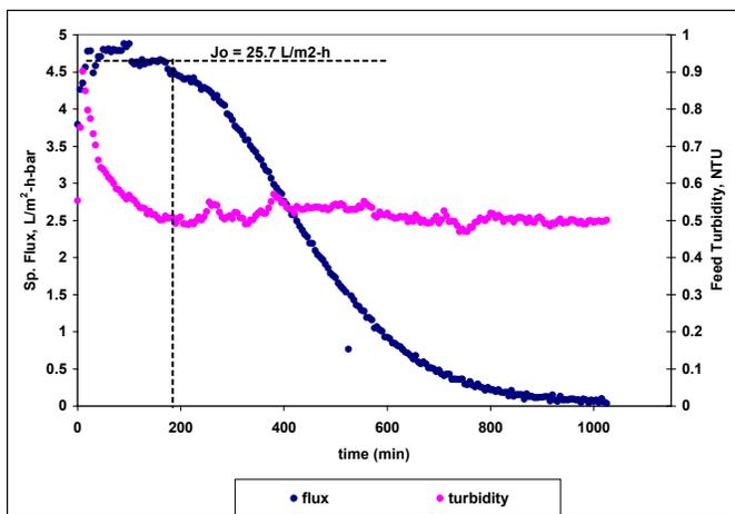
Figure 2: Induction time experiment with 0.03 M CaSO<sub>4</sub> and 0.06 M NaCl. P=10 bar, Q=100 L/m (0.7 m/s).
