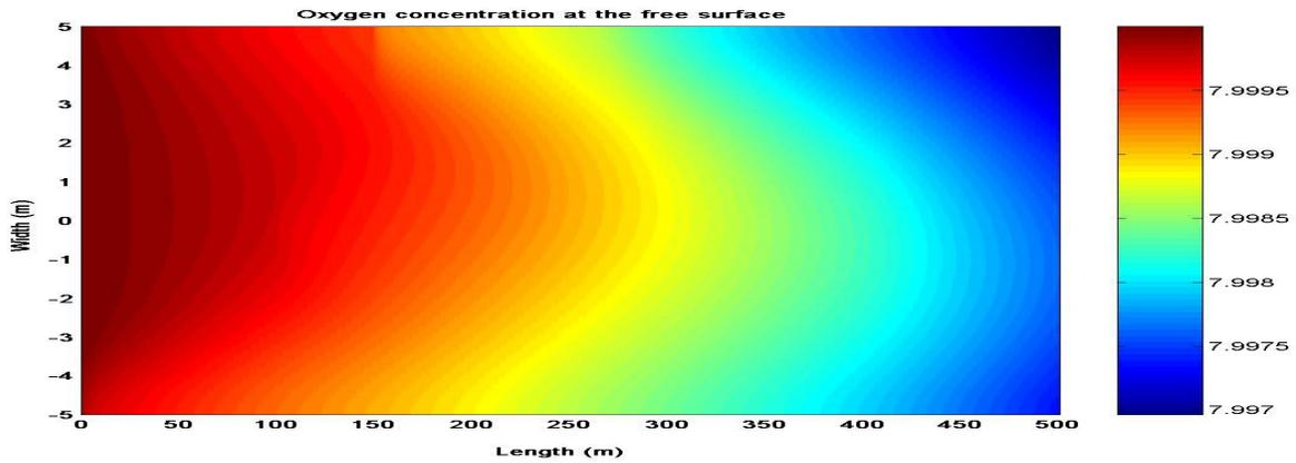
Figure 5: Contour plot of oxygen concentration at the river surface
