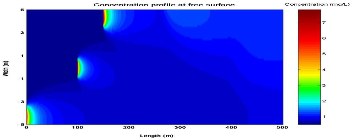
Figure 4: Contour plot of concentration at the river surface
