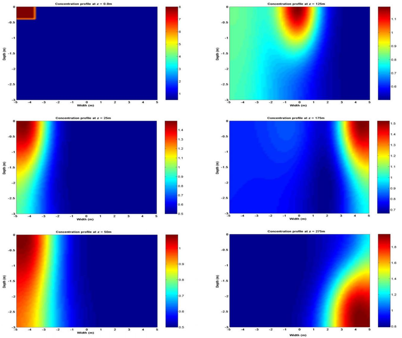
Figure 3 – Contour plots of concentration downstream from a continuous effluent release into a river
