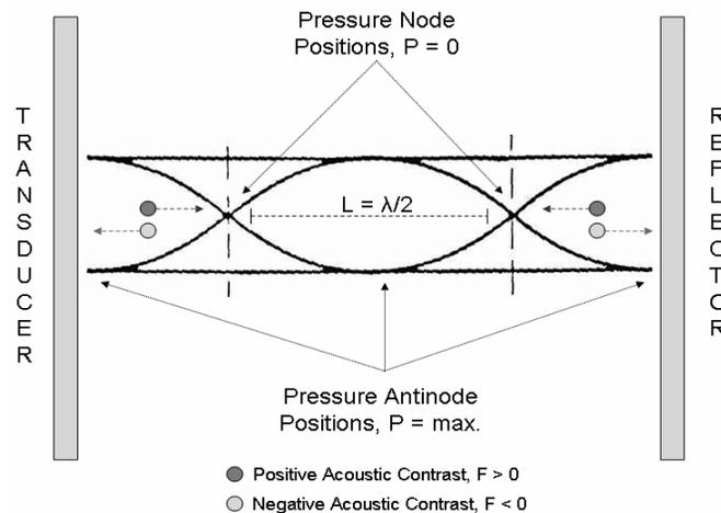
Figure 1 – Acoustic Chamber Schematic
