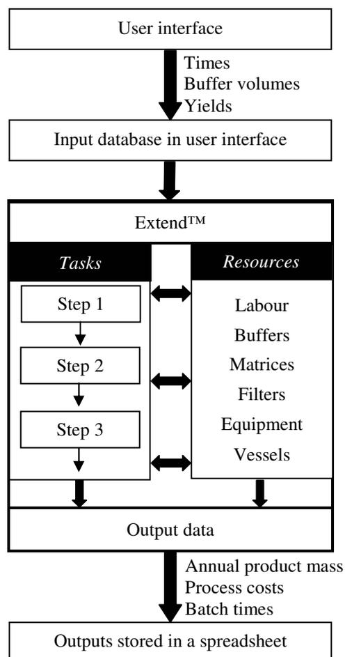
**Figure 2: Structure of the manufacturing model**
