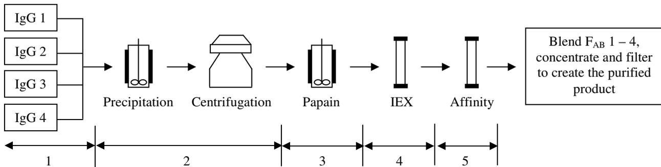
**Figure 1: Current process flowsheet, identifying the main unit operations: numbers specify groups of steps to which mass balance yield fractions were assigned in order to calculate the overall product yield. The process is operated separately for four feed sera, each containing one of the mono-specific anti-venom IgGs. Individual affinity purified batches of anti-venom  $F_{AB}$  are blended, concentrated and filtered to produce the final product**
